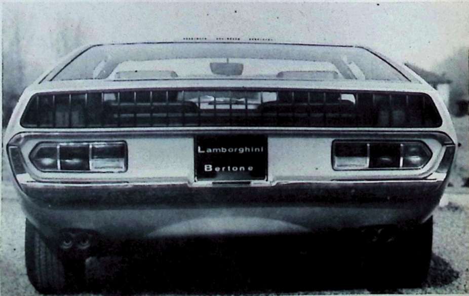
Bertone's newest masterpiece, his two plus two design for Lamborghini. The standard four liter coupe chassis has been lengthened by four inches. The Marzal idea car furnished much of the inspiration for the new production model.
