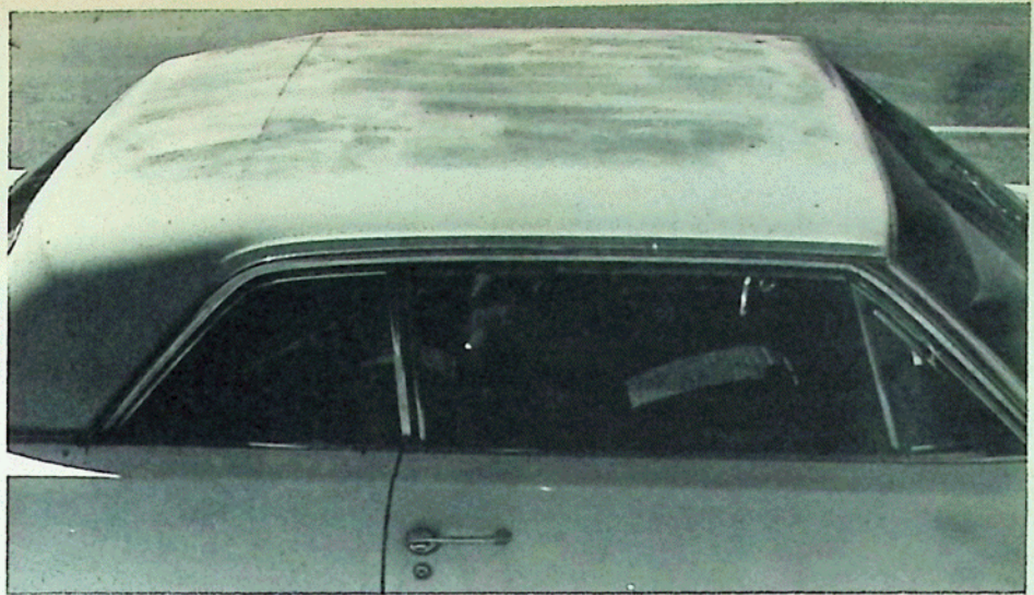
Exposed to the sun, paint on Chevrolet top deteriorates rapidly.
