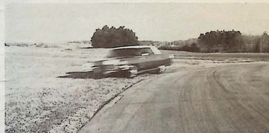
An automobile deliberately leaves GM test road to demonstrate how safe a highway can be if the roadside is cleared of obstacles and properly graded to provide a safe recovery area. It has been proven that a roadside can be made very safe with only 100 feet cleared and graded on each side, and only 25 to 30 feet would help considerably.
