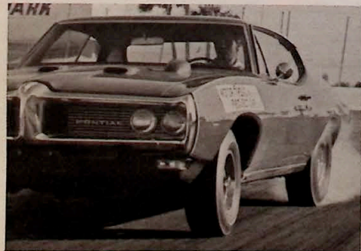
The crux of the Tempest Bobcat's modifications is the GTO's Ram-Air installation adapted to Tempest's 350-cu.-in. powerplant. That also means external changes like hood scoops.
