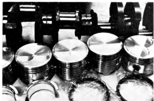
Joe Jill uses a dial indicator to check deck clearance with the unique Chevy rod setup. Piston pin location has been altered to work with hybrid rods. Crankshaft Co. made up the Dykes-ringed forged 12.4-to-1 slugs. Storm Crank reworked the arm.
