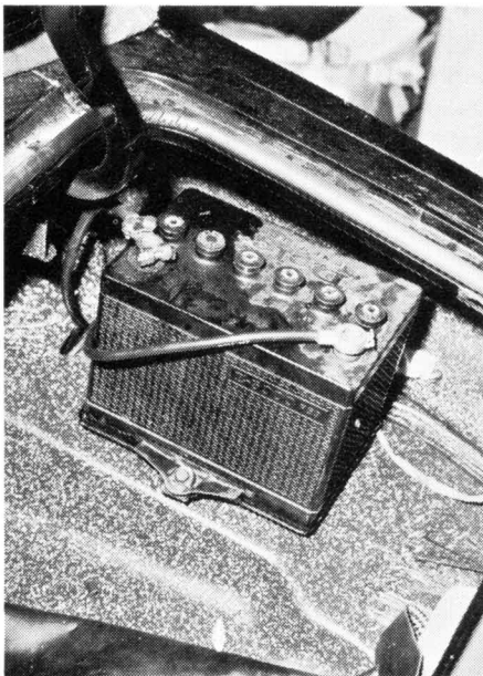
Street battery mounts in trunk over the right wheel. Truck battery will be used for comp.
