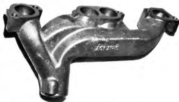
Left, Doug Thorley whipped up a set of special headers for prototype engine in a few days. They have new round port flanges with tuned tubing fitted to '68 GTO chassis. Right, exhaust manifolds are same basic layout as '68 but with inlets adapted to round-port heads.
