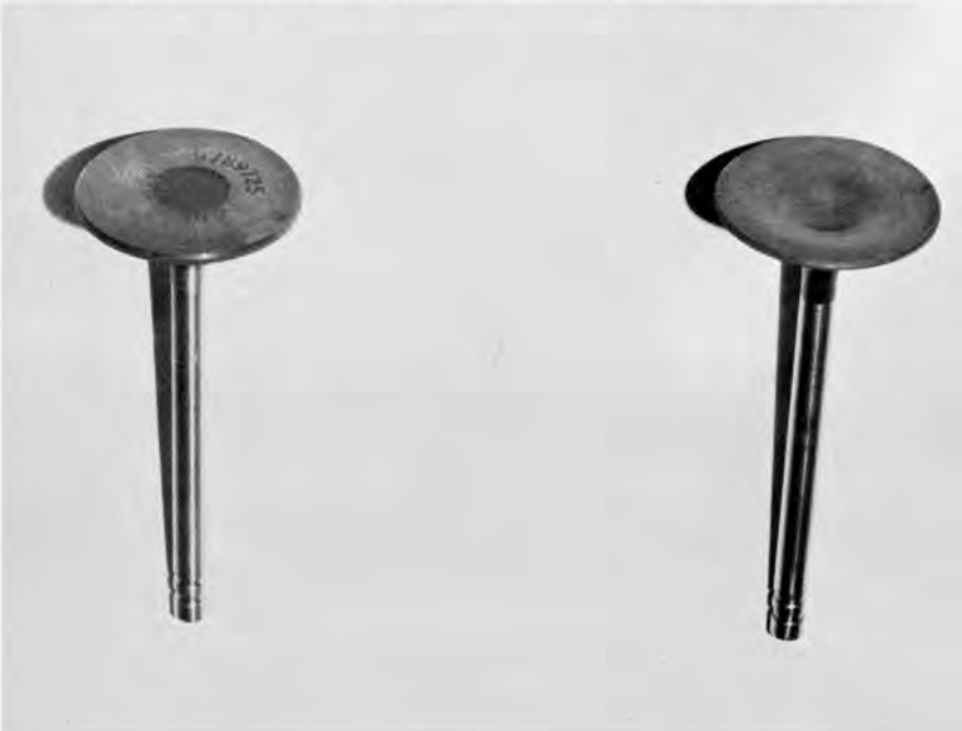
New intake valves have same 2.11 diameter but are tuliped to cut weight from 138 to 132 grams.
