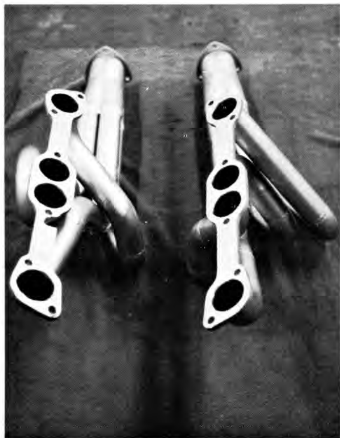
Left, Doug Thorley whipped up a set of special headers for prototype engine in a few days. They have new round port flanges with tuned tubing fitted to '68 GTO chassis. Right, exhaust manifolds are same basic layout as '68 but with inlets adapted to round-port heads.
