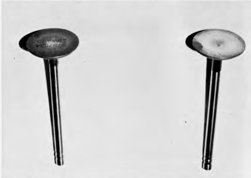
Exhaust valves are tuliped under head to reduce weight from 120 grams to 117 (valve on right).
