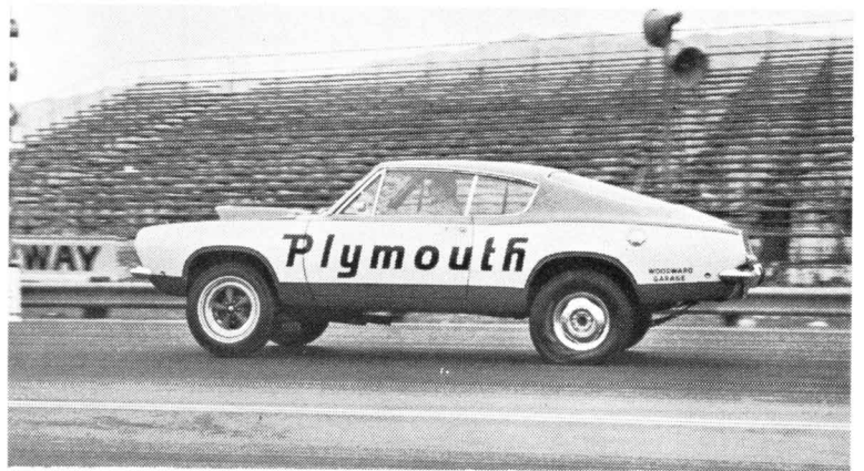
Powering the all-new factory Super/Stock Barracuda is a dual quad 426 Hemi with 12.5-to-1 pistons, solid lifter cam and steel heads and ram manifold. Car can be had with four-speed or Torqueflite. Up front there are fiberglass body components and a super light steel bumper. Car looks almost streetable. Hood scoop is functional. Gear chokes are 4.88 with stick and 4.86 with auto shifter.
