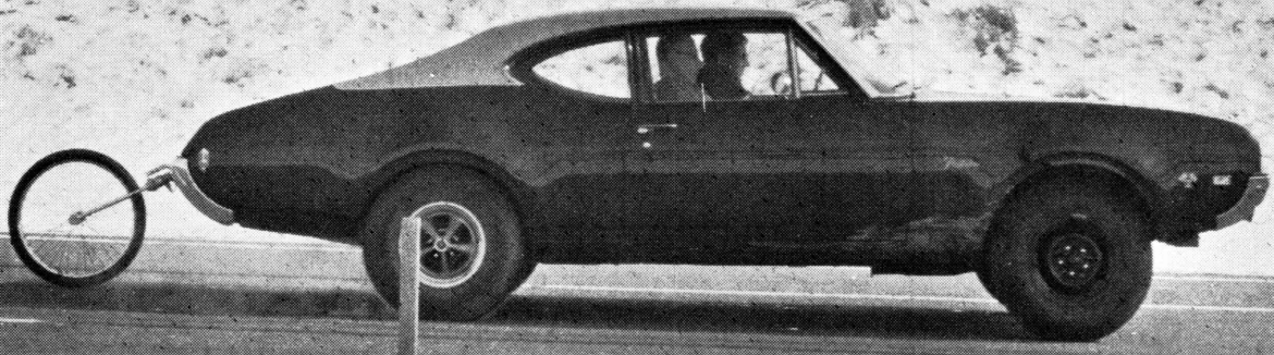
Author gets pushed back into his seat as the test driver burns out at 5500 rpm. Fifth wheel was used for accurate speed readings.
