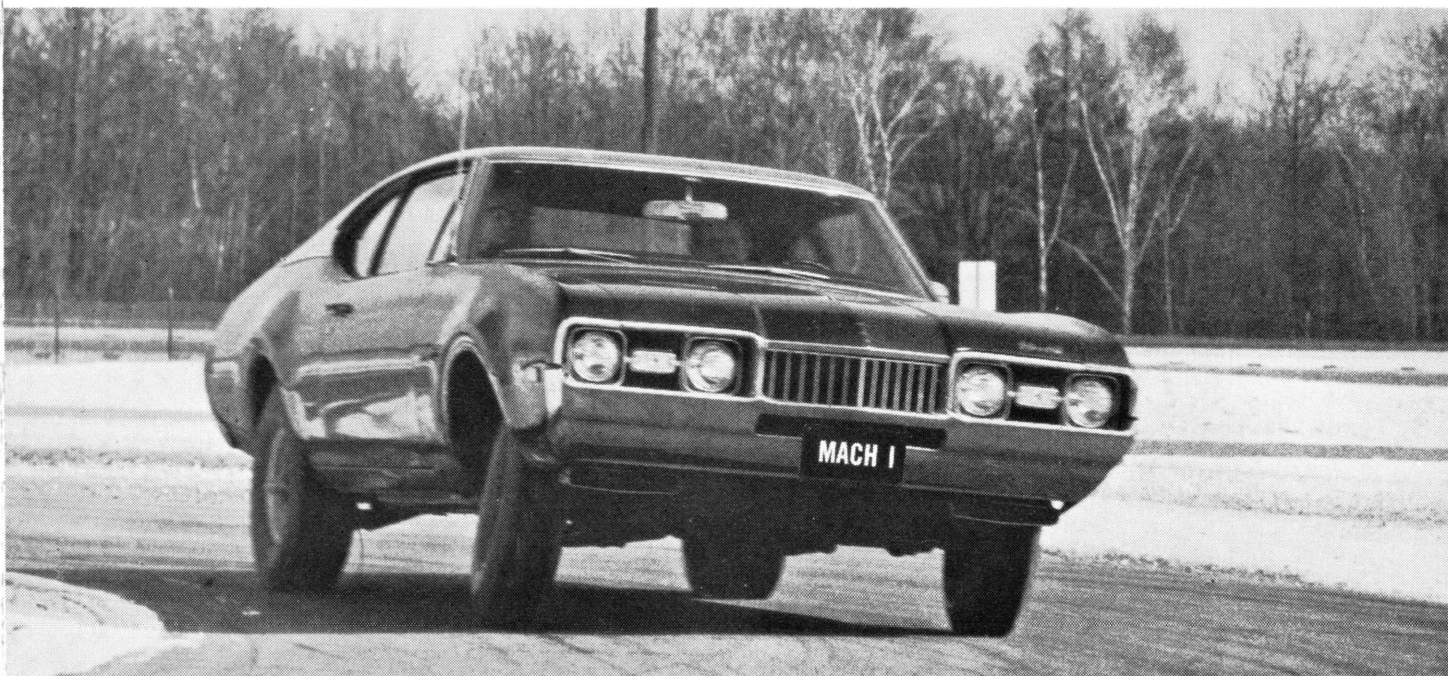
With slicks at the back end, 'Mach 1' Olds understeers on tight corners. Beefed heavy duty suspension is tops for street & strip.
