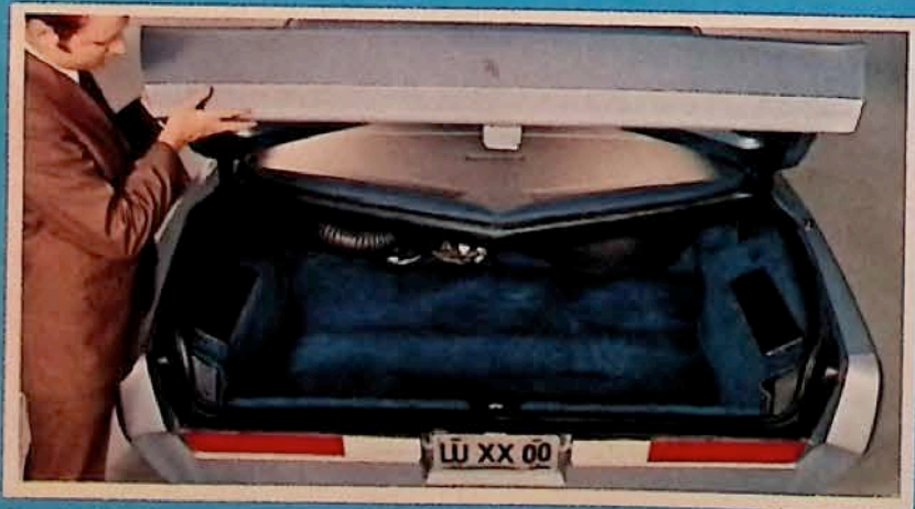
An electrically operated remote deck lid release gives a peek at the trunk. Remote release operates in "Park" only so lid can't accidentally open when car is in motion. Absence of rear frame members allows battery and AM-FM radio to fit in trunk.
