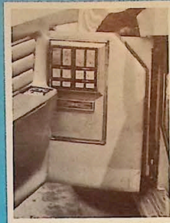
At the front of the left-hand door panel are switch touch plates set flush for safety. These control the driver's seat, window lifts, pedals, antenna, ventilation ducts, emergency flasher and trunk release. Flush mounted in the armrest are controls for the radio, each door has two sets of radio controls. Ash tray and lighter are also in the armrest.
