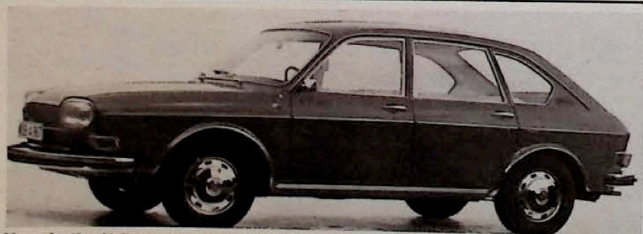
Here is the Volkswagen for which many have been waiting—the new Type 411. A new 1700cc engine with 75 hp powers the radical new sedan to a top speed of 95 mph. Wheelbase is 98 inches, overall length is 193 inches, and, best news of all is new front and rear suspension.
