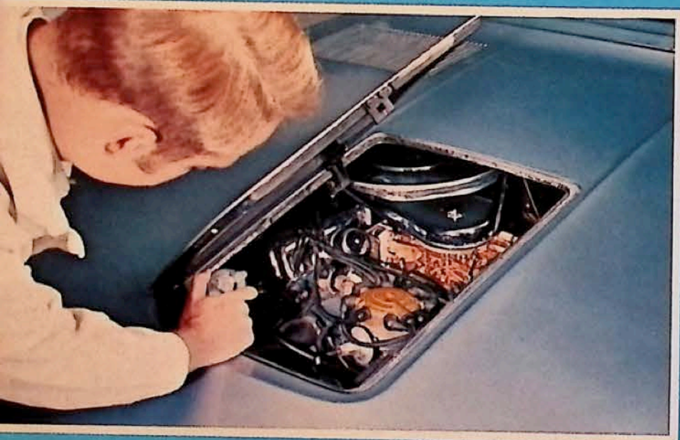
"Check the oil, sir?" A 14 x 24-inch side-hinged inspection hatch makes a neat hole in hood top. The hatch opening provides easy access for routine maintenance checks on coolant, oil, automatic transmission, carburetor and distributor and power steering.
