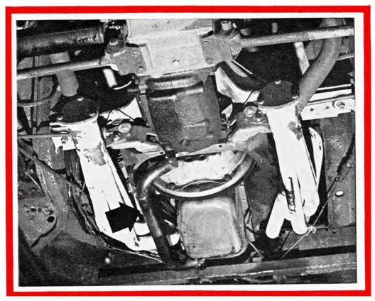
Ted Trevor stuffs a small-block Chevy into the back seat of a Corvair – retains the four-speed and independent rear suspension, all with no reverse rotation problems. The result?
