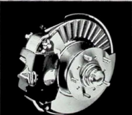
Cutaway shot of new floating-caliper-type front power disc brake. Single-piston design. Internal cooling fins rapidly dissipate heat. Availability depending on engine choice.
