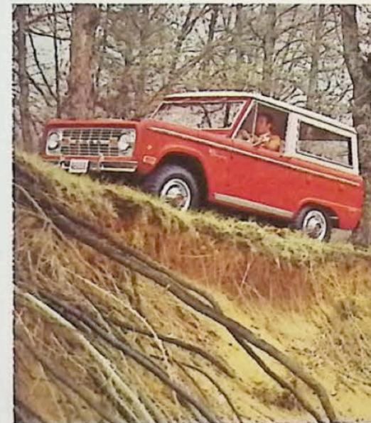
Go anywhere with a 4-wheel drive Ford Bronco. A round-the-town second car, or a spirited hunting and fishing companion. 4-wheel-drive traction sails you through mud, snow, sand. Smooth riding Mono-Beam front suspension; nimble 33 ft. turning diameter; powerful Six or V-8 engine up to 205 hp. Accessories include snowplow.
