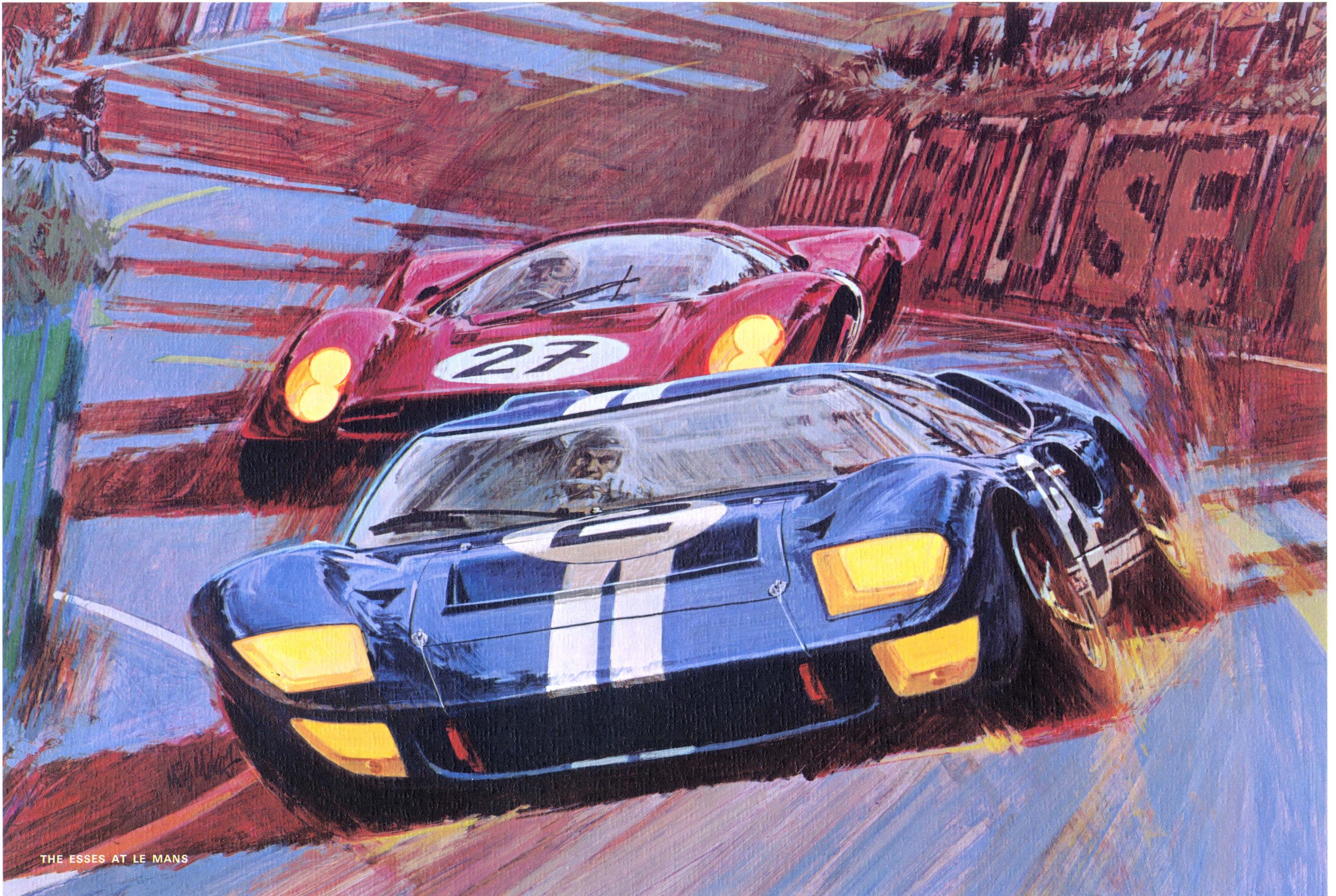
Ford GT Mark II. Unlimited sports car. American. Engine: overhead valve V8. Bore and stroke: 4.24" x 3.78" (108 x 96 mm.). Displacement: 427 cu. in. (6997 cc.). Compression ratio: 10.5 to 1. Brake horsepower: 485 @ 6200 rpm. Torque: 475 lbs.-ft. @ 4000 rpm. Clutch: 10" double plate. Transaxle: 4-speed synchromesh with limited-slip differential. Suspension: independent by coil spring, front and rear. Brakes: single caliper vented disc, front and rear. Wheelbase: 95". Overall length: 163". Racing weight (with 150-pound driver): 2832 pounds. One-two-three winner of 1966 24 Heures du Mans, Le Mans, France. Winning drivers: Bruce McLaren and Chris Amon. Distance: 3000.2 miles. New fastest lap record: 142.9 mph. Driver: Dan Gurney.
