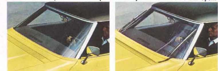
Hide-A-Way windshield wiper-washer system closed . . . and open.
