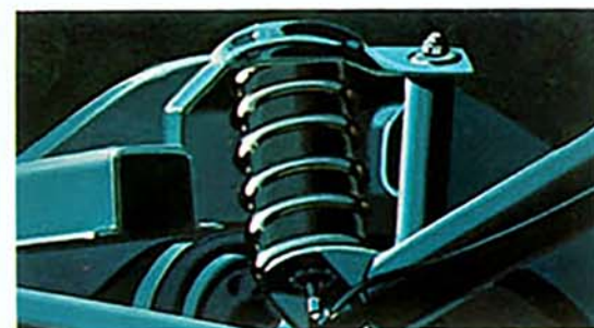
Automatic Ride Control. Pressurized air bags in each rear spring automatically help keep car at a constant height from the road and level regardless of load.
