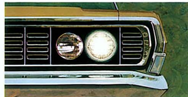
Retractable Headlamp Doors. Dual headlamps are concealed by grille door sections that retract when headlamp switch is turned on. Doors remain closed when parking lights are on. Standard on LTD, XL, Country Squire.
