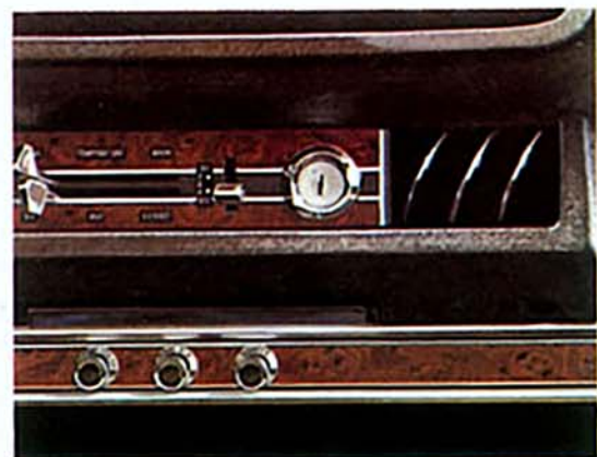
Comfort-Stream Ventilation. A better idea that adds extra comfort. Fresh air enters through grille on the cowl, circulates without noise or drafts, forces stale air out even with all windows closed.
