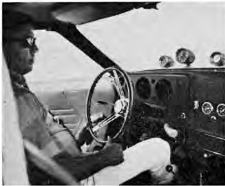
RON ROOT'S SUPERSTOCK Javelin charges off the line during qualifications for the Super Stock championship, above. He trailed the Dodge factory's best, but lost in the third round. Below left, Root checks his instruments. The Javelin has extra gauges in the panel, and atop the cowl, in the driver's line of vision. Fuel pick-up tank, below right, has the pick-up below the tank proper, so gasoline will be forced into the line during acceleration.
