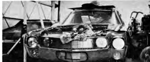
AMX PREPARATION was still underway at this point. Front view, above, shows extra lights for night driving during endurance runs. Below, engine builder Jim Ward puts final touches on the supercharged AMX engine.
