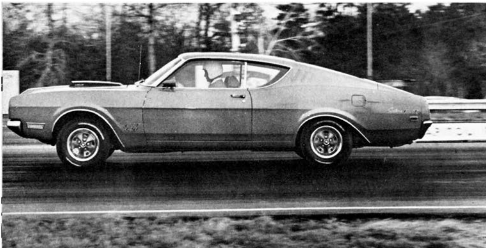
TOP—Polyglas tires helped, but off-the-mark starts were hampered by loss of traction as soon as power overcame the tires. Note the lift of the front end upon mashing the throttle! ABOVE—Emblems on the side tell you that this Montego is different from all the others on the block. Here we go to a best of 13.99-103.92. The SelectShift C-6 trans shifted crisply and flawlessly during entire twenty passes.
