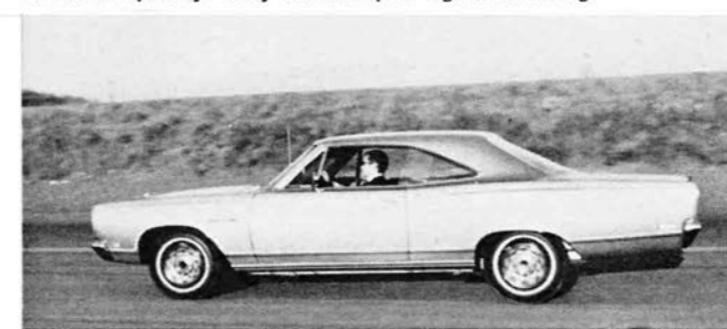
LEVEL Plymouth doesn't illustrate stiff springs. The rear wheels lock so quickly that the fronts can't do any work.
