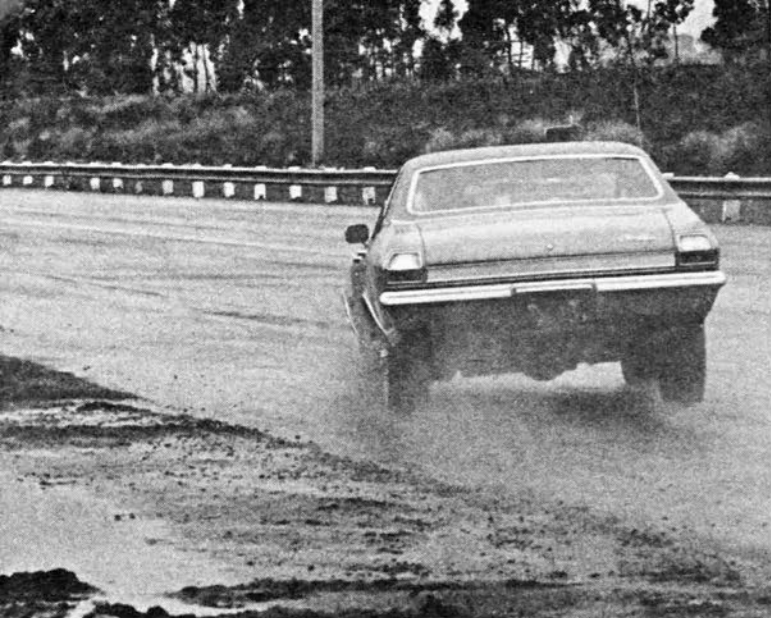
SCARY MOMENT came when Chevelle locked one wheel during brake test, and spun the car half-way around. The flaw was the fault of the one car, but Chevrolet's high-boost power brakes magnified it. The light pedal is difficult to modulate.
