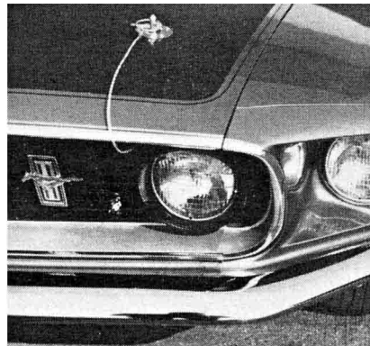
PINS keep the hood closed, and nylon-covered cables keep the pins in place.
