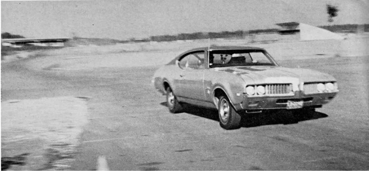
SUDDEN CHANGES of direction were the W-31's meat. Strong suspension allowed the test drivers to put the car through a sharp left, then a sharp right, at high speed, without loss of control. Most family cars, and some Supercars, won't do it.
