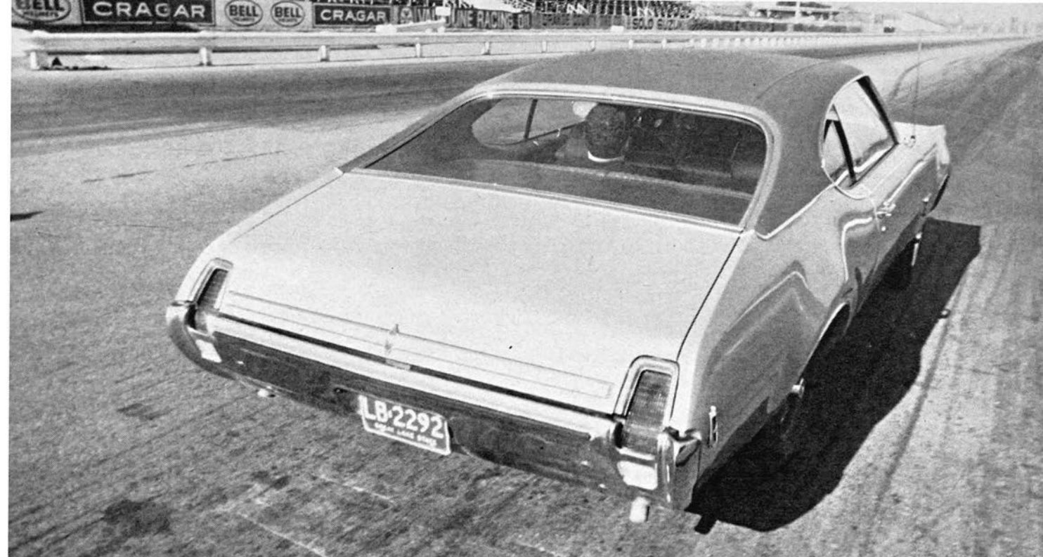
RAKED ROOFLINE put the rear window as close to the rear-seat passenger as it could be. As a personal judgement, the testers didn't feel that the optional (and expensive) vinyl roof covering blended with or improved the lines of the body.
