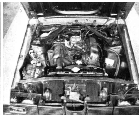
(Above) Base engine in the Cougar, the 351 fills the engine compartment to apparent capacity. Note the large amount of space between grille and radiator. (Left) Entering curve at speed, Cougar hugs road, is predictable and easy to control. Kicking rear end out is a matter of choice. Ride isn't overly hard.
