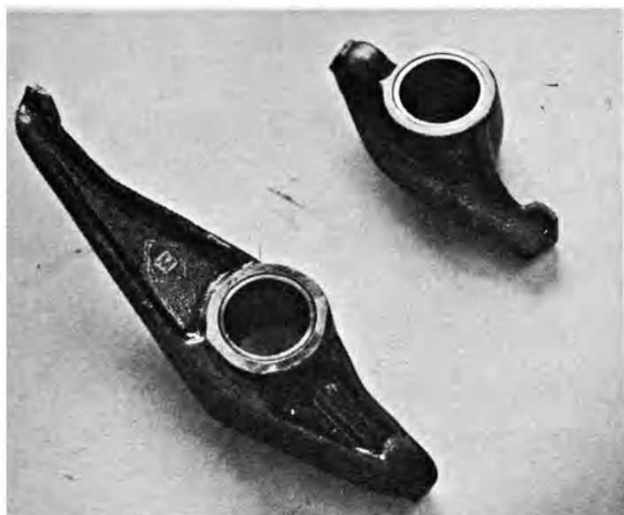
Rocker arms are forged high-alloy steel for maximum strength.
