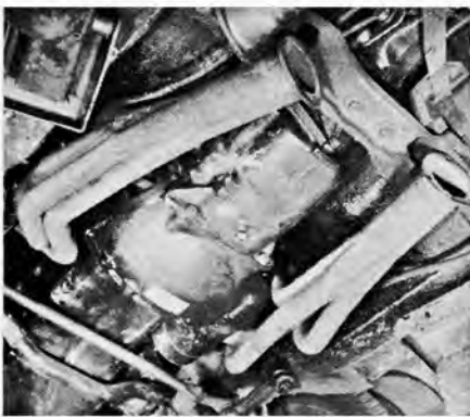
Slick-shifted four-speed close ratio trans is used with a light weight solid hub clutch disc.
