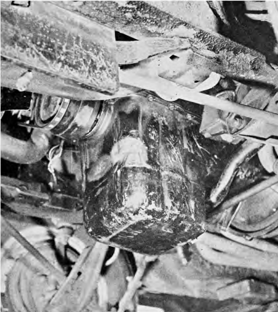
Deep sump oil pan holds eight quarts plus one quart in the oil filter for a total of nine.
