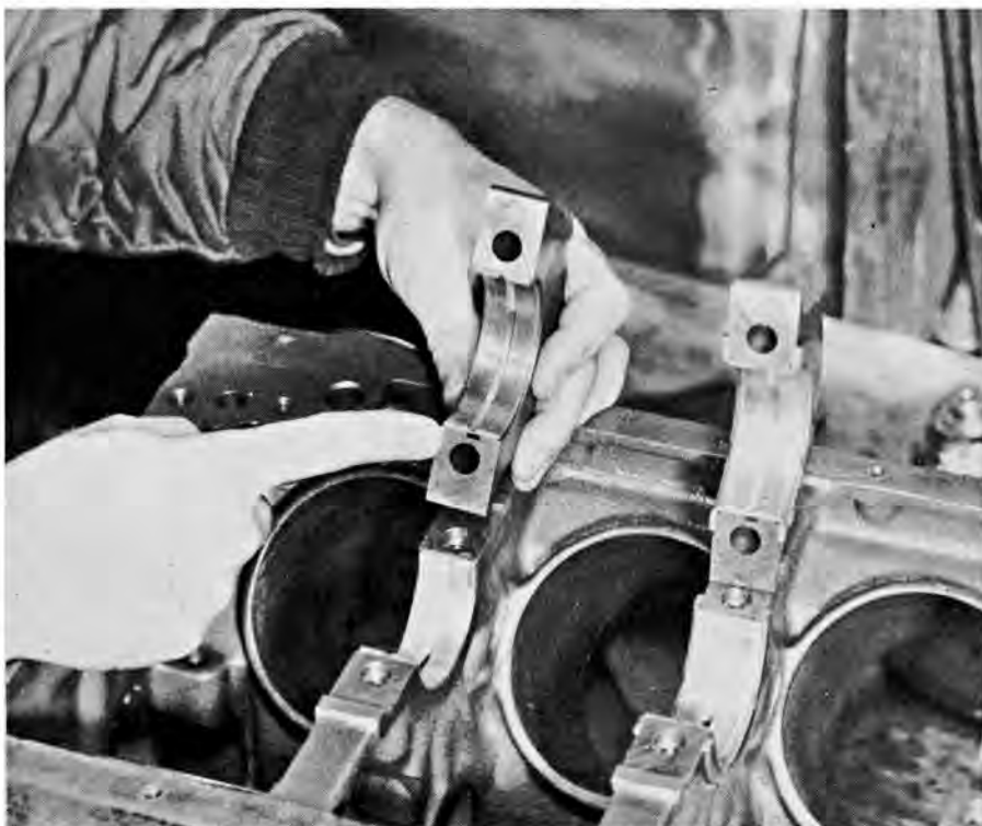
Retaining tangs from an extra set of main bearing shells are used in the main bearing caps.
