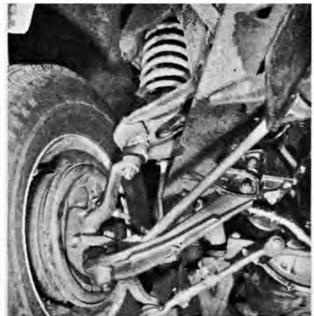
Top, Shelby intake manifold had squared off galleries. Bottom manifold used by Bob Corn has smoother transitions. Below, front end leveled by adding spacers at ball joints.
