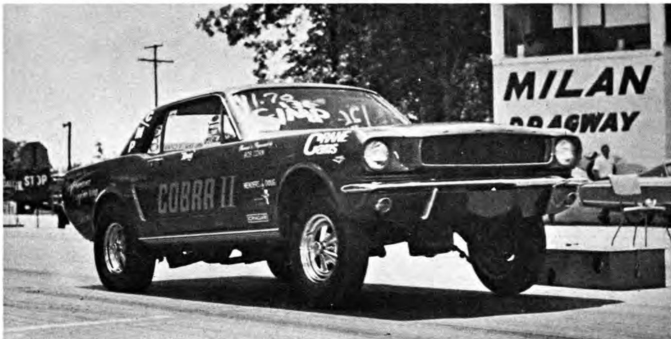
For instant traction, you need all the weight on the back and so Bob keeps his front wheels just barely touching the ground.
