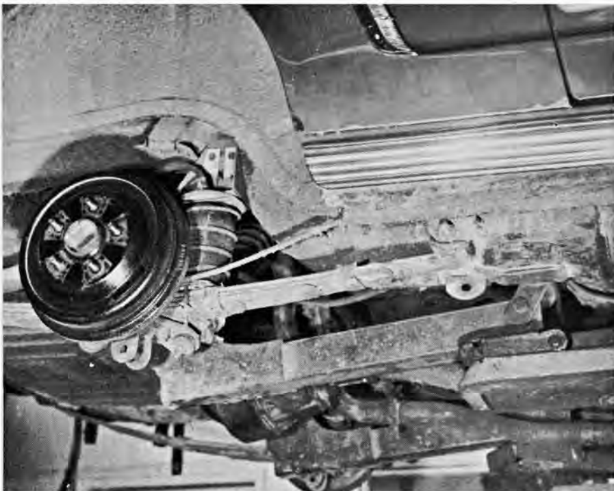
The stock springs are supplemented by 35-inch traction bars, air lifts and helper springs.
