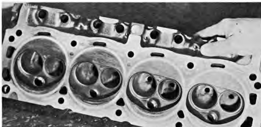
Experimental ignition system is transistorized. Positive lock clamps hold down the distributor cap. Drive for mechanical tach was added. Shelby-American did extensive work on combustion chambers and increased valve seats. CC's are made up by using piston pop-ups.
