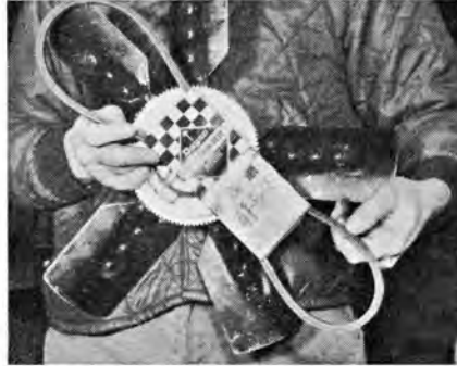
Dayco Racing Belt stands up well to the 8000 rpm shifts. Prestretching could be the reason.
