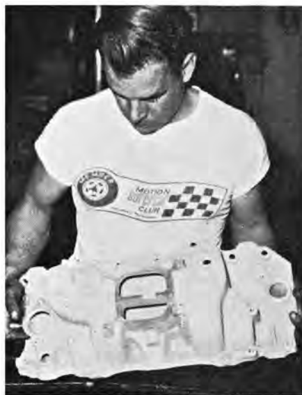
Edelbrock manifold is designed to use Holley three and four-barrel carbs on small port heads.
