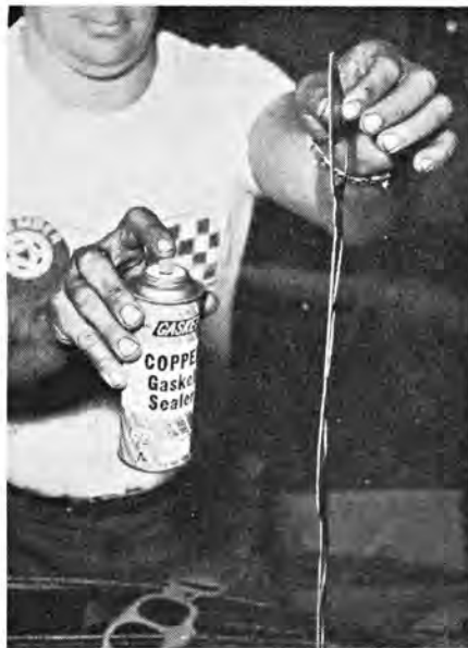
Intake gaskets must be sprayed with sealer to guard against manifold vacuum leaks.
