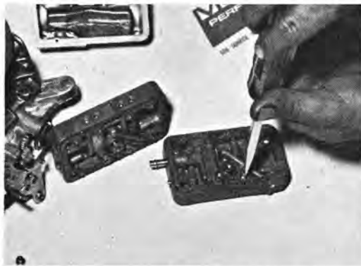
The hot setup quad is the 780-800 cfm Holley quad as used on the old 425-hp 427 Vette. Jetting should be altered as outlined in the text. Carb linkage arm should be checked for full throttle operation and drilled if necessary for the cable hookup.
