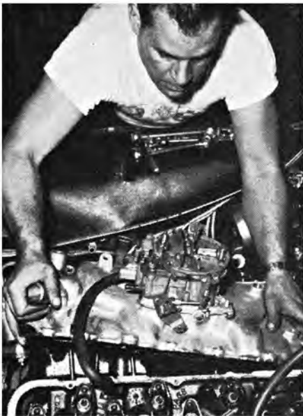
First disconnect all fuel and vacuum lines and remove the stock carburetor and manifold.
