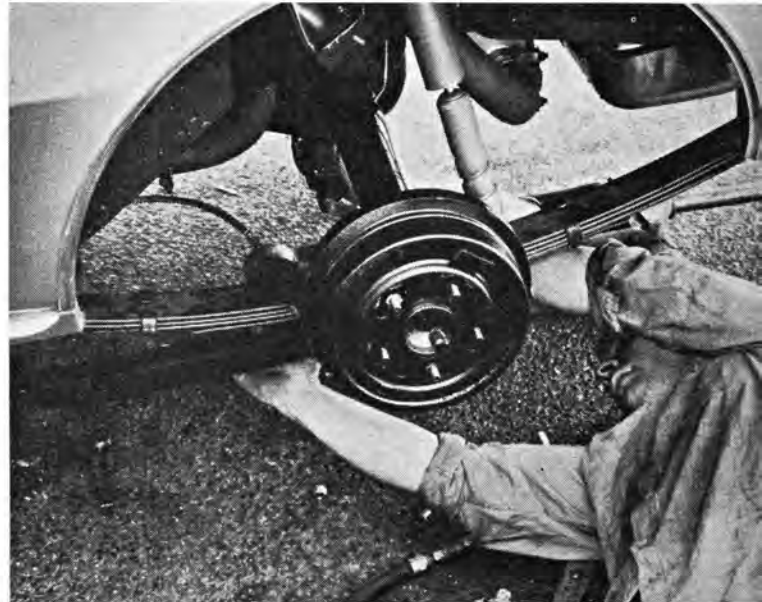
Multi-leaf rear springs should be fitted with traction bars.
