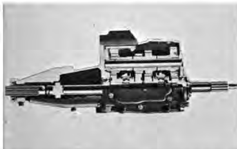
Ford cars ordered with overdrive get the T-86 unit. It's n.g. for HP machines.
