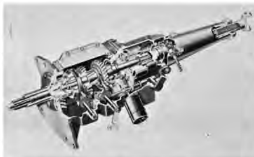
Sectional view of GM Saginaw all-synchro three-speed. This trans is the base for GM's '66-'69 Saginaw Four.
