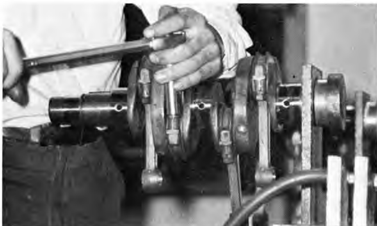
Sklaski torques the matched rods to the Revmaster "B" 74 mm crankshaft. Extra care goes into the assembly of the engines slated for racing.
