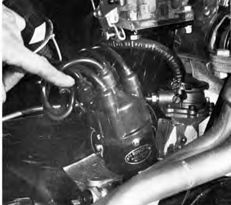
A centrifugal advance distributor takes the place of the stock vacuum actuated item. Sklaski sets them up to reach full advance at 2500 rpm. A total of 38 degrees of advance is used with 10 degrees on the crank and 28 degrees in the distributor.
