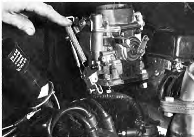
Recommended carburetion for the 85 hp engine is a Zenith 32 NDIX. Rochester and Stromberg carbs have been tried but on the dyno the Zenith was found to be superior.
