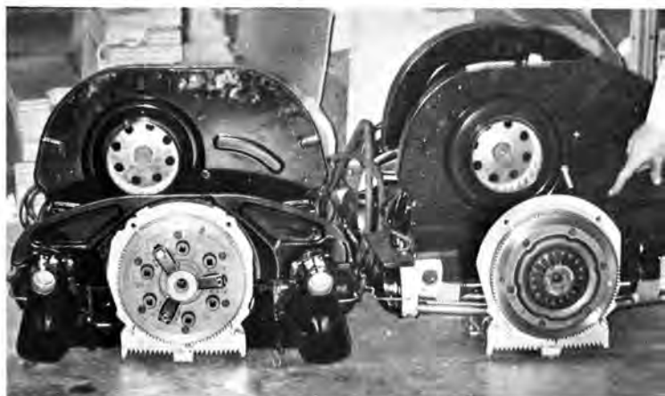
To harness the horses Revmaster recommends a 180 mm clutch assembly. This can be either a Luk or Hausermann. Here the assembly is compared with a stock unit on the left.
