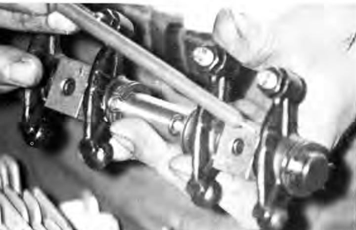
Rocker arms from the 1500 series engines are identified by the two marks on the end shown here. The 1500 arms have a ratio of 1.1-to-1 which is a 10 per cent increase in cam lift over those from the 40 hp series.
