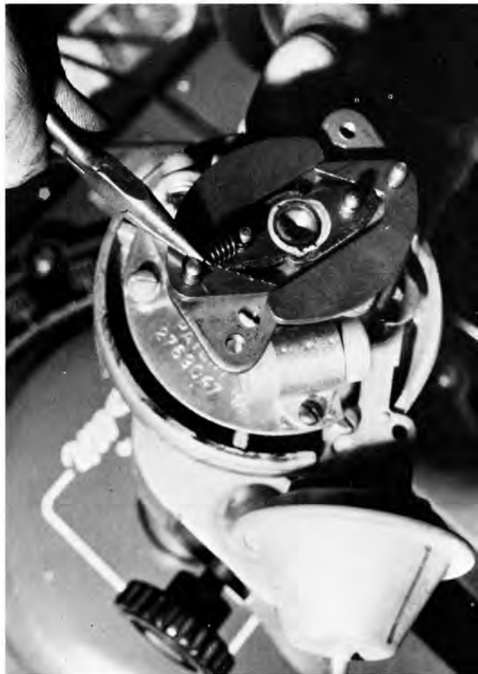
To change the advance curve, Harold replaced the stock distributor springs with the much lighter Iskenderian ignition springs. With a little experimenting the advance curve can be tailored to fit any situation.
