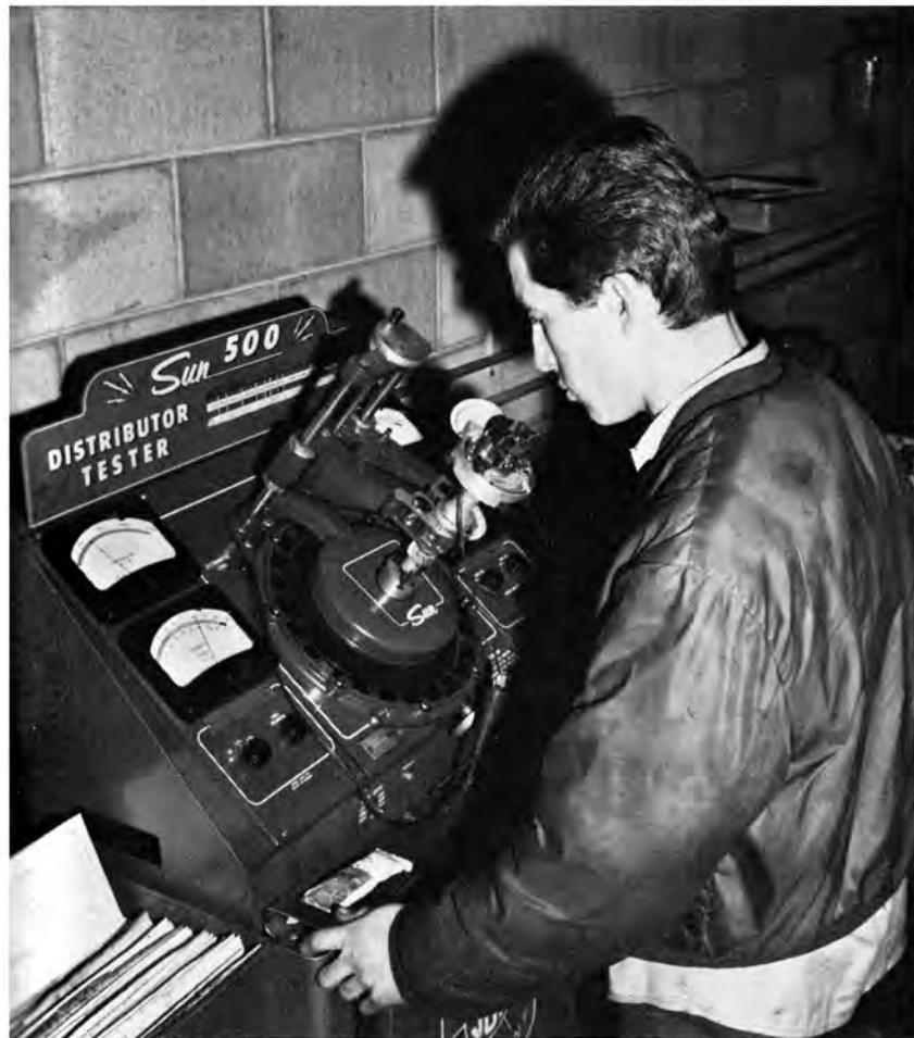
Harold Lawrence checked out the Judge's distributor on a Sun 500 t4ster, then replaced the advance bushing to limit initial advance to 10 distributor degrees. He also set up a new advance curve so that total advance was reached at 2500 rpm.
