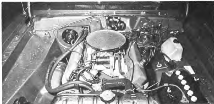
440 mill rests in the Dart's engine compartment with little room to spare. Big inch with gobs of torque makes machine one of the strongest runners to be found.
