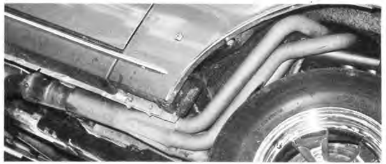
Hooker Headers exit through the fender wells into 3" collector, 18" long. H.P. increase is high, as 440 mill needs to breathe at the top end. "Western" style snubber has 3/4" clearance from floor pan, controls wind-up.
