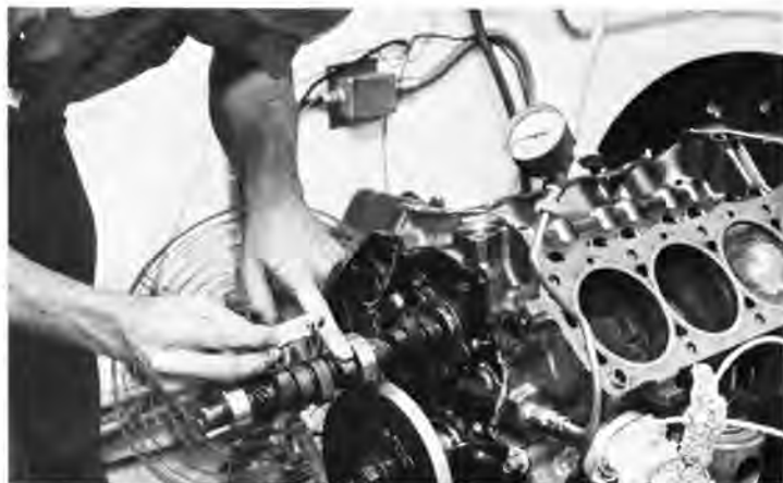
Linton applies Assembly Lube to Crane H232/310 CompuCam as a safeguard against wear during break-in. Lifters should also get a liberal coating. Wilder cams will be tested in Part 2.
