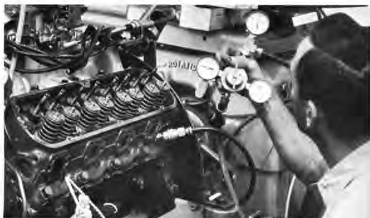
After each dyno run, each cylinder was leakage checked with Rockair tester. System shows up problems not revealed by a simple compression check. Valve seats caused initial woes.
