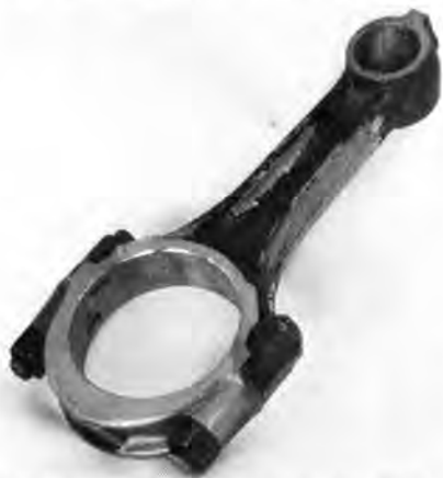
Ford's forged connecting rods for the 302 street version are an improvement; bigger 3/8" rod bolts are employed for ruggedness.
