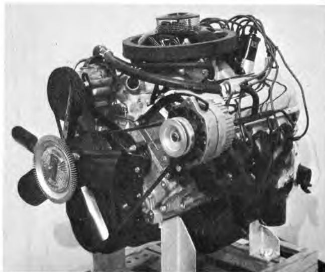
Much-talked about, long-awaited all-aluminum ZL-1 engine is factory rated at 430 horses. New “Rat” saves 175 pounds over cast iron counterparts and 100 over aluminum headed L-88.
