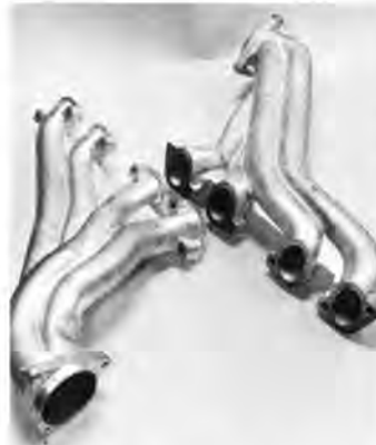
We said it was a racing engine! Stock individual iron exhaust castings are slick, but heavy.
