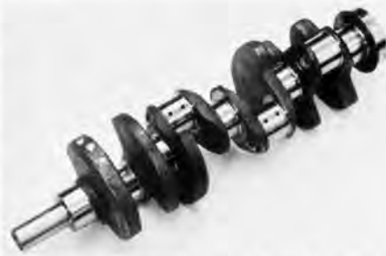
The crank is forged steel rather than iron, another Ford first as far as production small block equipment is concerned.
