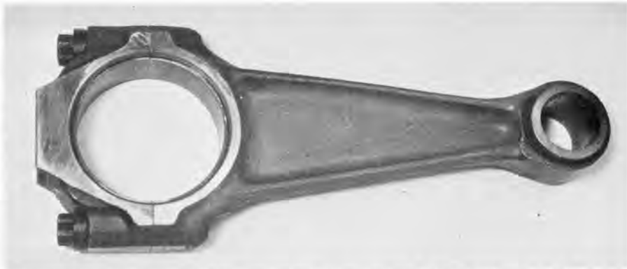
Beefy-looking connecting rod is all-new for production engines, but was first used in 1963 in NASCAR Stock Car competition. Rod should help "wild Indians" live longer.
