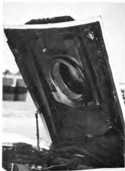
Functional rear scooped hood pushes air through plenum chamber to polyurethane sealed and filtered carburetor breather.
