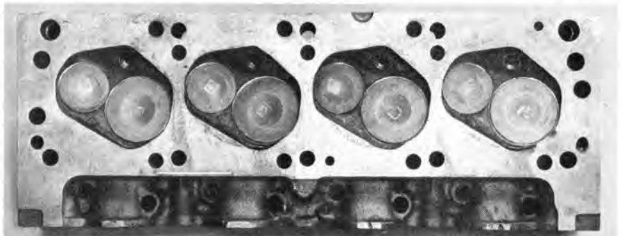
Land of the Giants. Combustion chambers house whopping 2.23" intake valves and 1.71" exhausts. Canted valves permit more water jacket cooling around exhaust valves.
