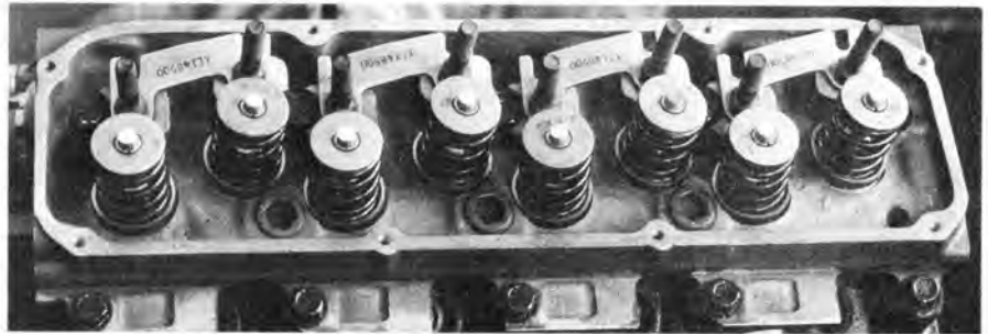
Inclined valve approach is apparent with staggered spring setup, rather than earlier in-line technique. Hardened steel pushrod guide plate keeps everything in its place.
