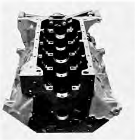
SOHC uses same basic block as 427 wedge. Oil system must be checked, some passages enlarged, others blocked.
