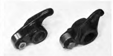
Chromoly exhaust rocker, left, is must for blown fuelers; gas SOHC's can safely use lightened, reworked stockers though.
