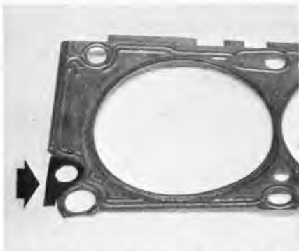
Stock 427 steel shim head gasket is one to use, but small velumoid insert must be used to seal around the drain-back hole.
