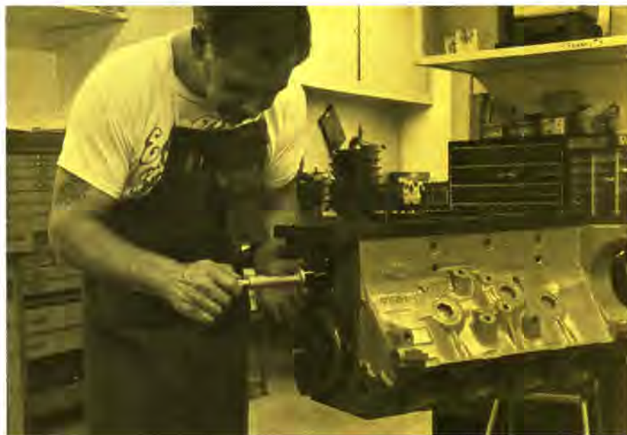
With main caps and Milodon steel lower end support torqued in place, Federal Mogul main bearings are each checked in two places with three-anvil hole mike. This gives accurate i.d. measurement and check of concentricity. Desired main clearance is .006.
