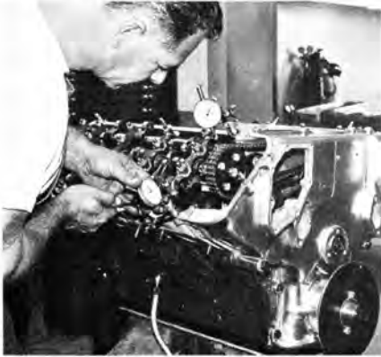
Specially fabricated fixtures hold dial indicators in proper position for checks of valve timing and camshaft placement.
