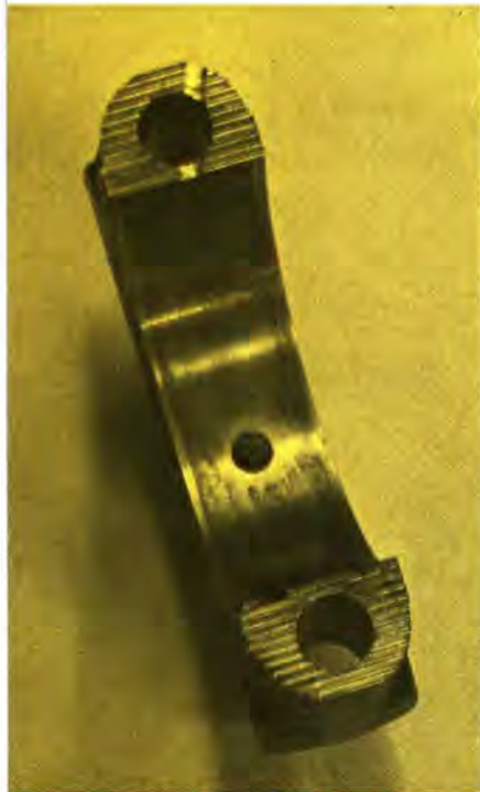
Small oil groove on outboard side of rod cap helps lube lower cylinder. Bearings must be drilled to fit on locating pin.
