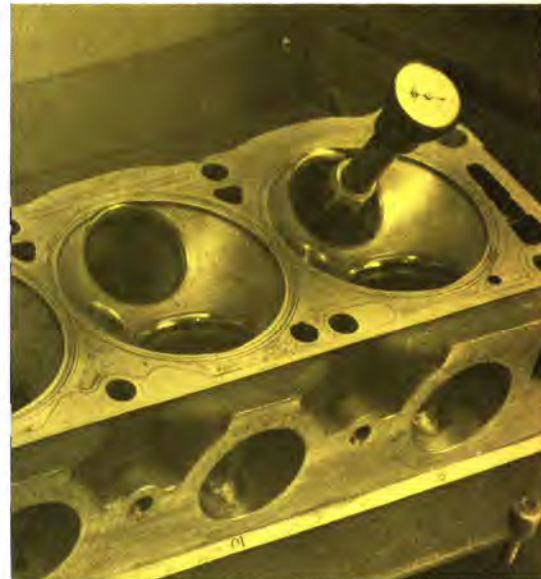
Small dial indicator is used to check concentricity of valve seats with guides. When using aluminum heads, Ed treats the exhaust ports with heat-reflective coat.
