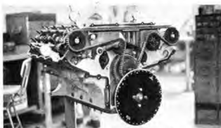
Six foot timing chain drives the Crane 612A cams. High rpm stretch necessitates use of the different initial cam settings.
