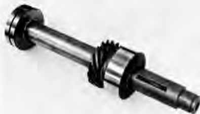
Shot peened accessory drive stub rides in #1 and #2 cam bearings; oil pump and either mag or injector pump run off it.
