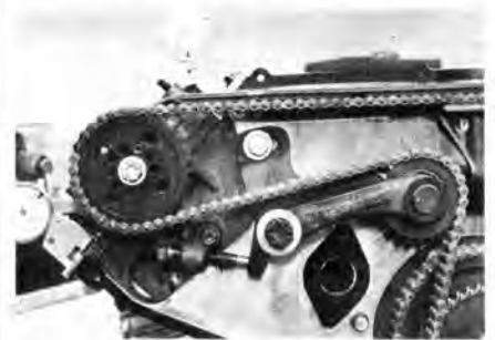
Proper tightening of chain tensioner is vital. Continuously turning engine over during tightening helps eliminate slack.
