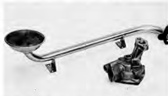
100 psi of oil pressure is supplied by a '57 Ford pump. Pickup feeds at rear of modified pan and sits 1/8" off bottom.
