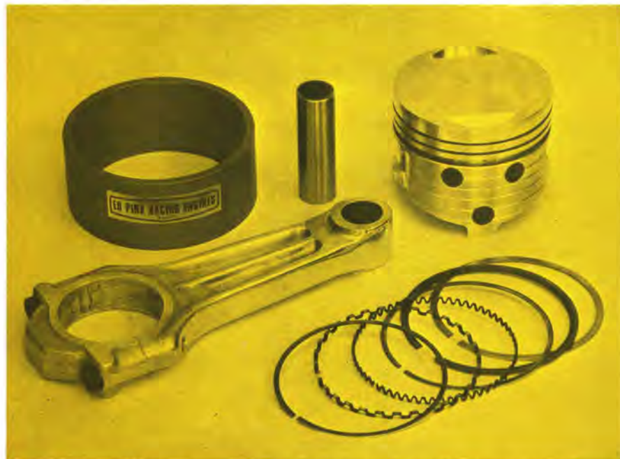
Pink starts with M/JT aluminum rods, completely remanufacturing them. Pistons are by Forgedtrue, running 8:1 compression, and normally four buttons per side are used to steady each in bore. Top ring is Forgedtrue Step-Seal, second and third are Pedrick.
