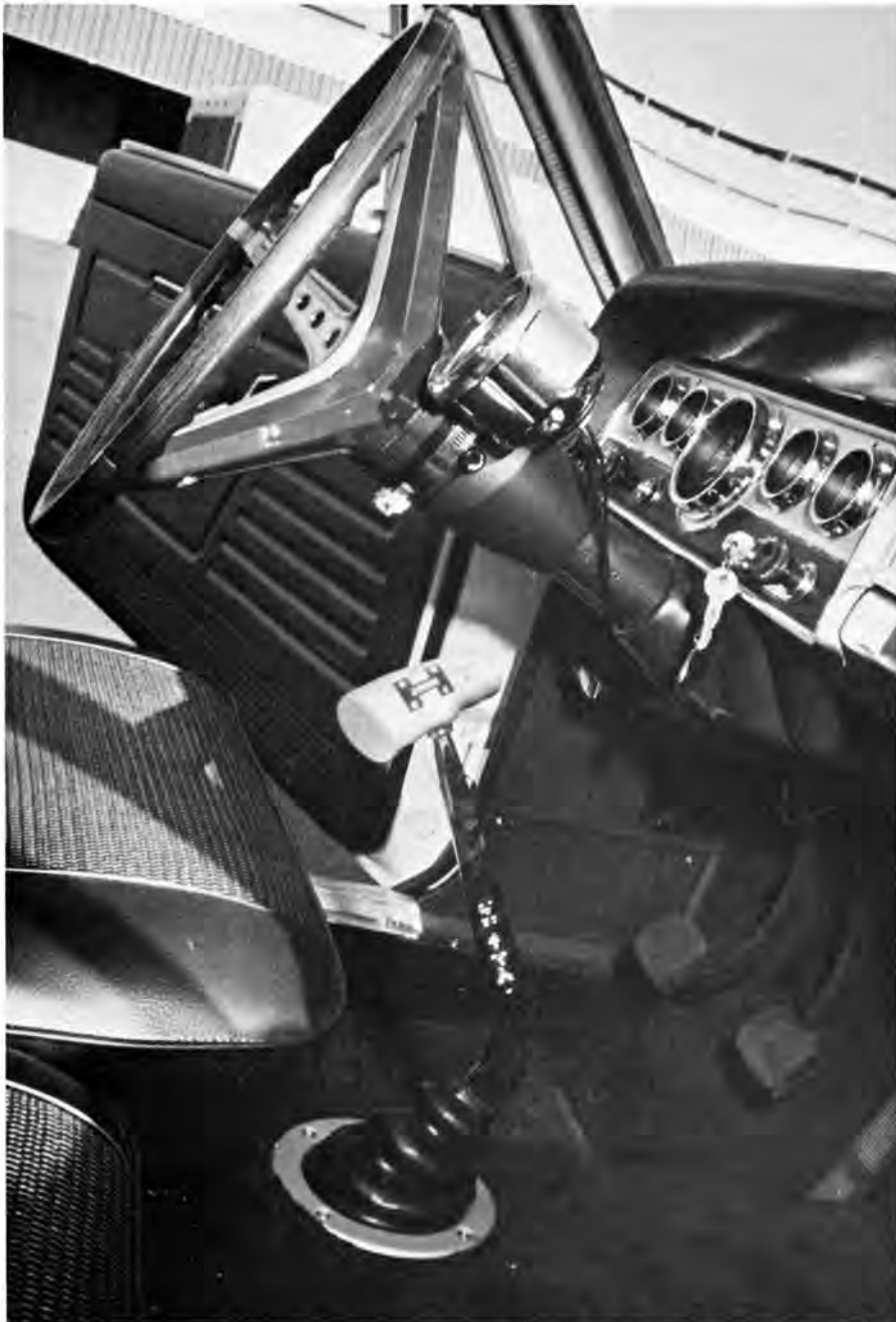
The interior, basically stock Rambler with gauges for speed, fuel level, and temperature, (idiot lights show loss of charge or oil pressure) has been supplemented with a Sun tach and Hurst production line shifter.
