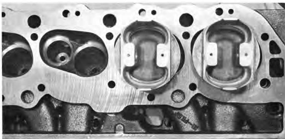
Chevrolet's 396/427 "semi-hemi" has unique combustion chamber with tilted, staggered valves that may set pattern for the industry. It combines advantages of hemi and wedge layouts. High power in small, light engine. This is the big-port high-performance version with forged pistons.
