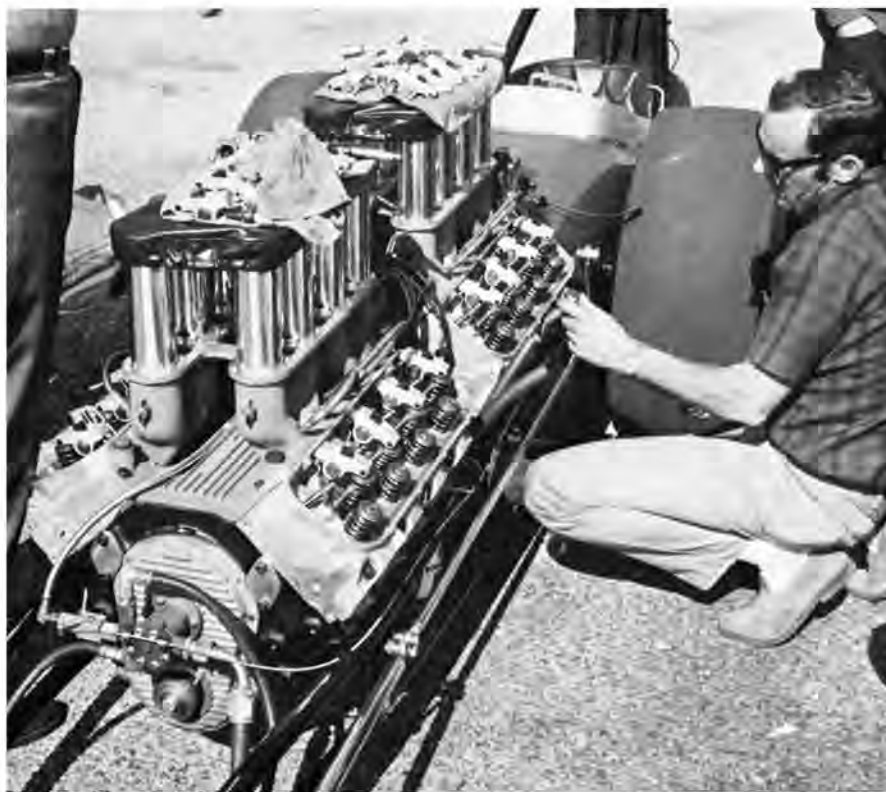
The L-78 version of the 396 engine is used in this dragster. Aluminum heads on the 427 engine designate the powerful L-88 powerplant and now a ZL-1 engine — all aluminum — is Chevy's new bid for supercar supremacy. Over 600 hp with an engine that weighs in the area of 500 pounds.
