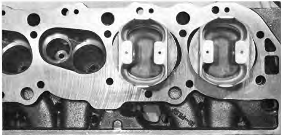
Chevrolet's 396/427 "semi-hemi" has unique combustion chamber with tilted, staggered valves that may set pattern for the industry. It combines advantages of hemi and wedge layouts. High power in small, light engine. This is the big-port high-performance version with forged pistons.
