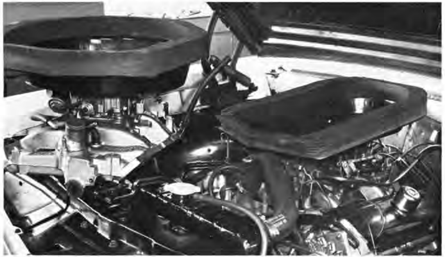
Pontiac pioneered with "Ram Air" system for the '65 GTO. First system used hood scoop feeding cold air to foam-sealed air box around Tri-Power carbs. Picture shows Tri-Power Ram Air system on GTO, with '67 Ram Air Quadrajet setup alongside. Good for 10 to 30 extra horses!
