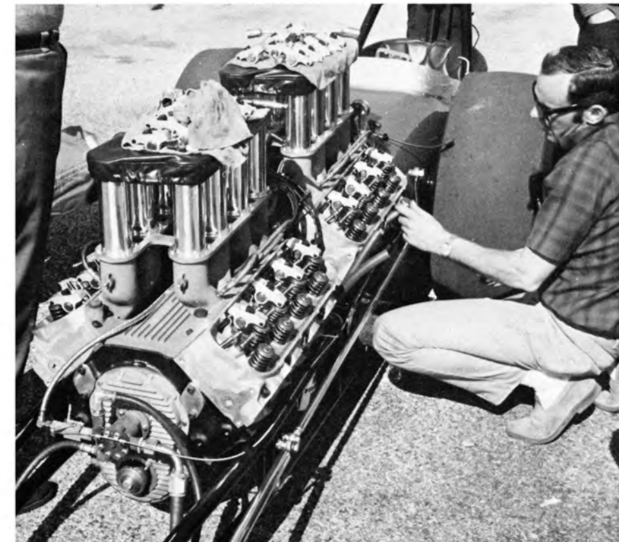
The L-78 version of the 396 engine is used in this dragster. Aluminum heads on the 427 engine designate the powerful L-88 powerplant and now a ZL-1 engine — all aluminum — is Chevy's new bid for supercar supremacy. Over 600 hp with an engine that weighs in the area of 500 pounds.
