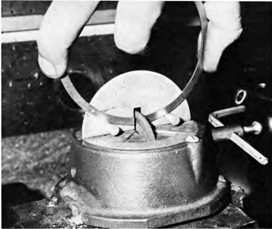
Butt-gap (end-gap) resizing can be accomplished by careful perpendicular filing of ring ends or by use of "trick" gappers like the one shown here.
