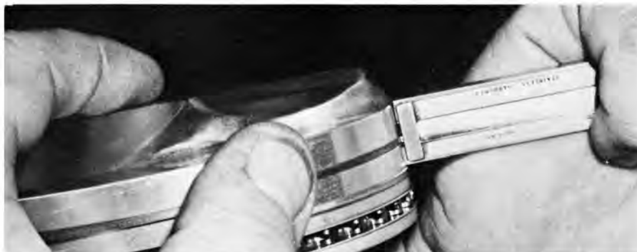
Ring groove depth is especially important for performance type ring jobs. Generally, ring manufacturers give specifications for their particular ring design. Look on the instruction sheet (if all else fails).
