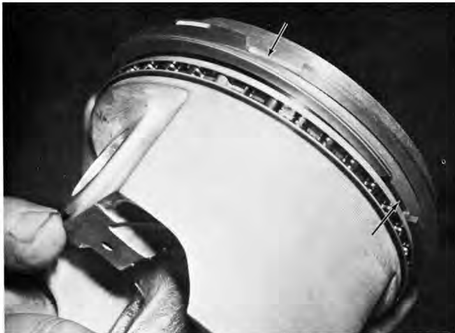
Staggering of ring end-gaps is also important, usually involving a separation angle of 45-50 degrees (on one of the piston's thrust sides).
