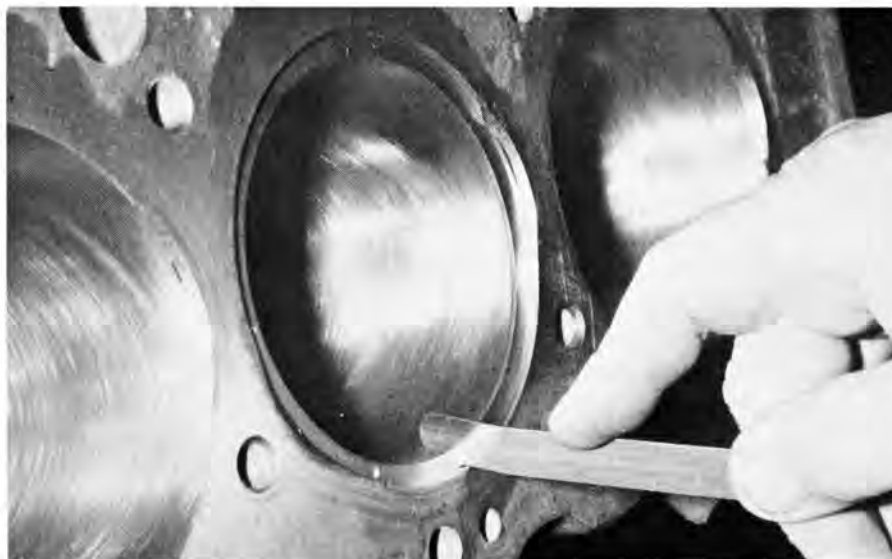
End-gap check is made by installing ring in cylinder (near top) and measuring with feeler (strip) gauge.
