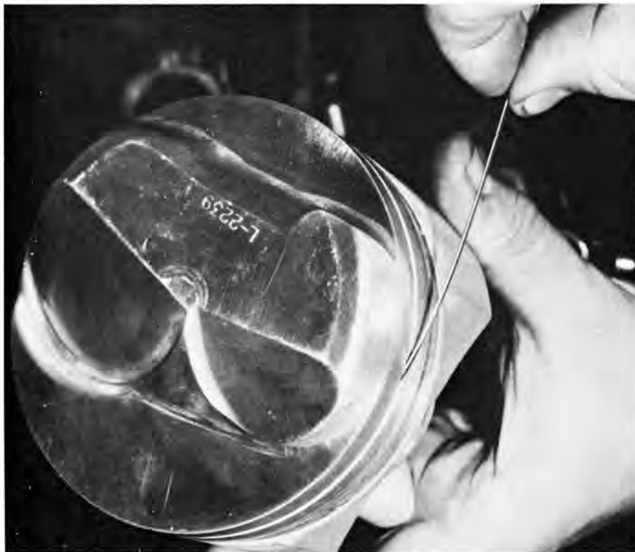
Addition of extra ring expander stock (under compression) rings is a performance-type trick designed to further aid high cylinder pressure seal.
