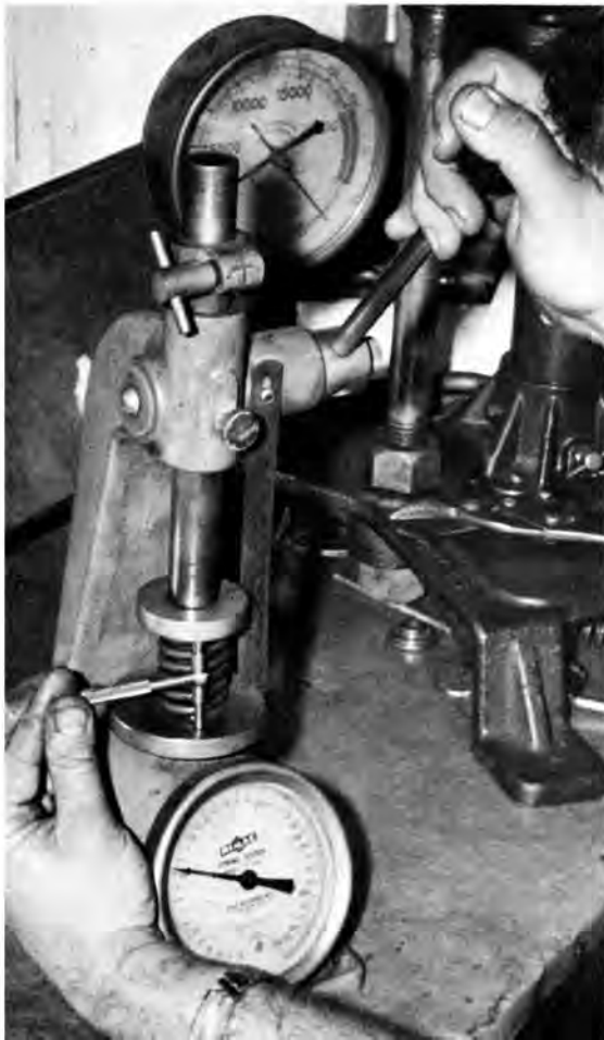
Spring pressure reading can be correlated with recommended height of installed spring. Exact seat pressures can be determined and spring pressure uniformity checked (with low or high springs being discarded).
