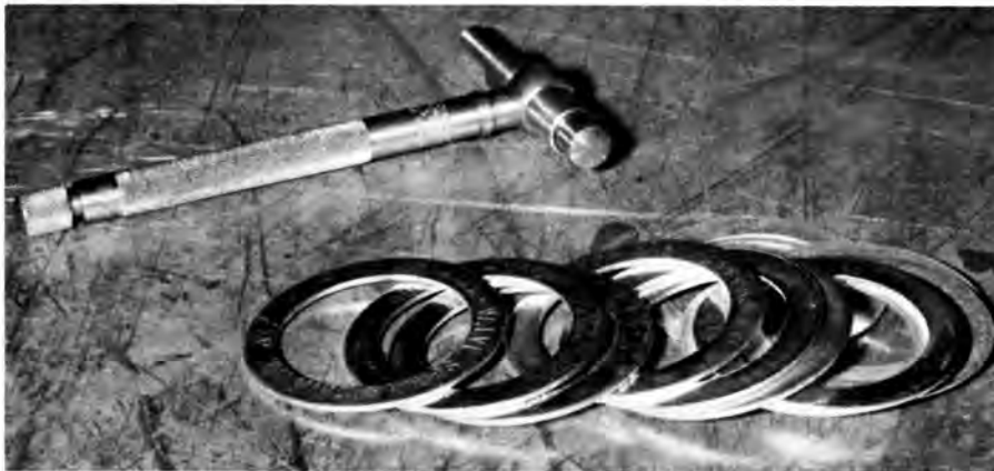
Assortment of spring shim material is available and should be used for accurate spring height on assembled head. Snap gauge is well worth the money.
