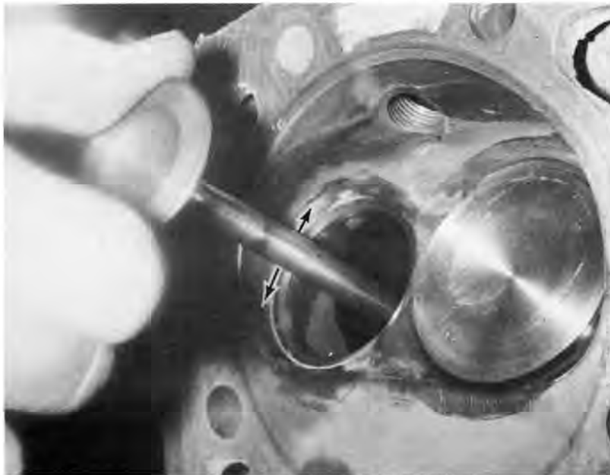
Wobble check of valve in guide will indicate need for installation of oversized valves (stems) or reconditioning (knurling, inserting, etc.) of guide bores.
