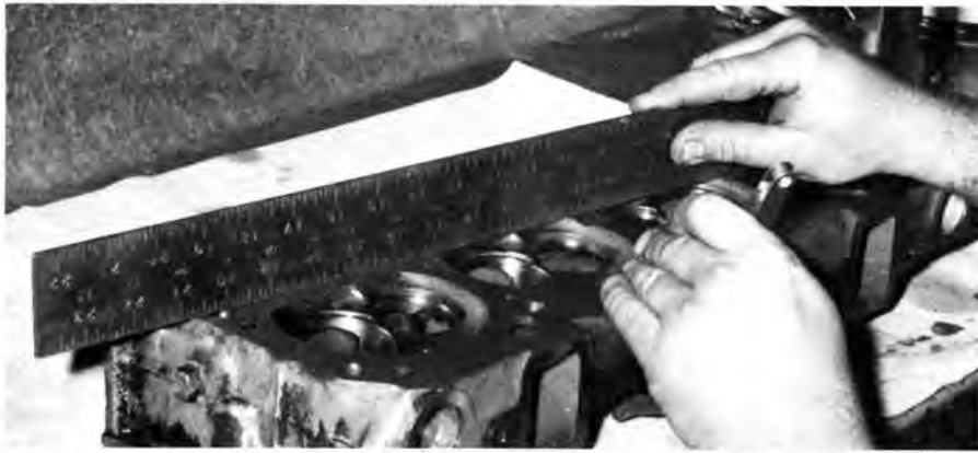
Head warpage check (during valve job) can cure possible pressure leakage problems later after job is complete. Surfacing or slight head cut is needed only to remove gasket etch or to correct excessive air gap (in excess of 0.008-0.010-inch) measured with strip gauge between head surface and straightedge.
