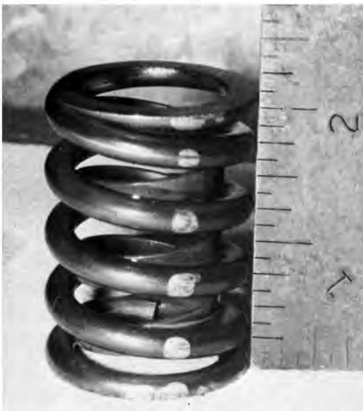
One necessary spring check is for "cock". On a level surface, spring should stand "square" (perpendicular) with base. Variations here make a spring subject to scraping, since it operates with less than its designed pressure.
