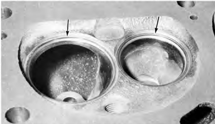
Position of performance type valve seats is normally at extreme edge of valve and is usually of a width ranging from a hair-line out to .030-.040-inch (depending upon whether the seat is an intake or an exhaust).
