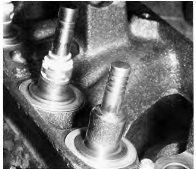
Valve guides (especially intake valve guides) should be fitted with some sort of seal (Perfect Circle, etc.) to retard oil drain-down and lack of guide/stem seal during use of high lift (high valve-scrub) camshafts.
