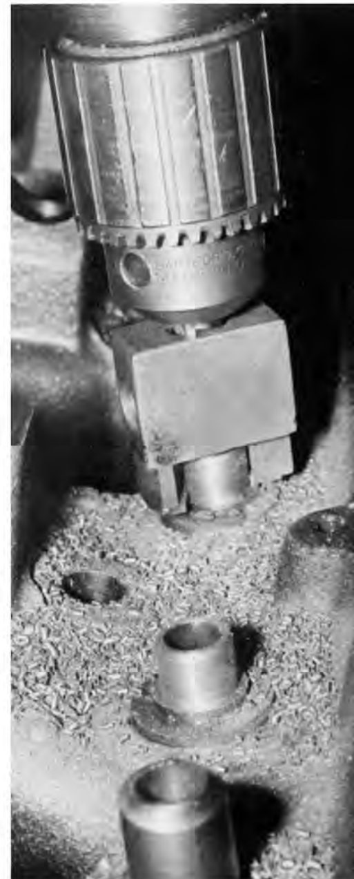
Wobble check of valve in guide will indicate need for installation of oversized valves (stems) or reconditioning (knurling, inserting, etc.) of guide bores.
