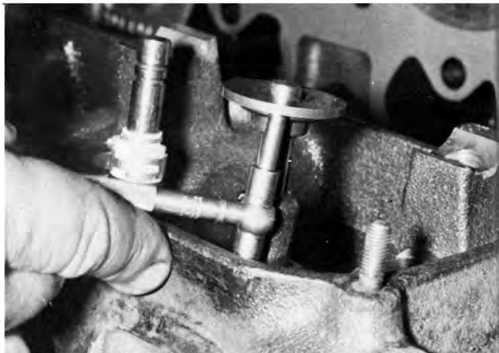
Spring "stack" (installed spring height, valve seated) is fundamental to correct valve performance. Use of snap-gauge on installed spring retainer will indicate shim material (if any) needed for proper spring height.
