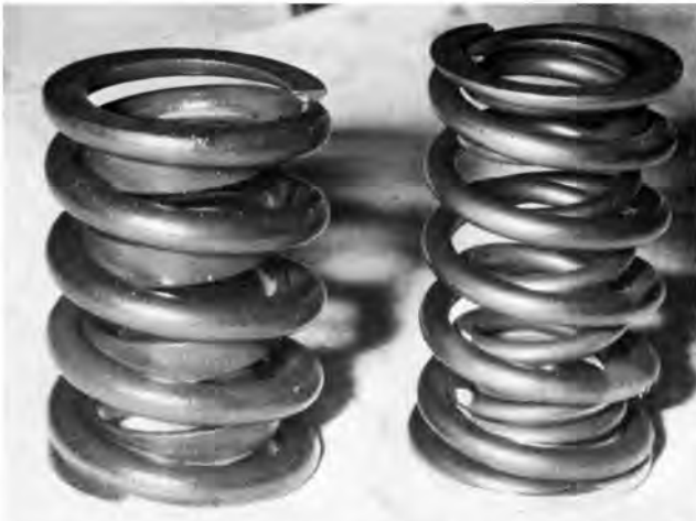
Performance valve springs can be of either or a combination of these two shown. Flat steel coil is a harmonic surge damper (springs have resonate frequency points in their cycling range) which adds very little spring load; other spring incorporates counter-wound inner spring for additional spring pressure. Some super-duty springs incorporate both harmonic damper and inner spring.
