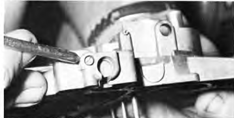
Adjustment of secondary air valves involves turning spring-loaded screw at right-front corner of carburetor top. Opening rate should correspond to pattern mentioned in story.
