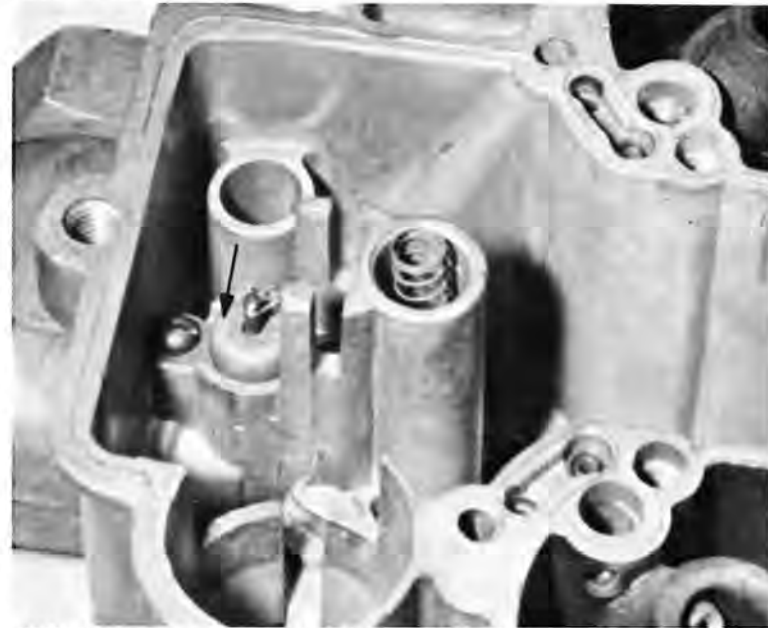
With bowl member removed, needle and seat become exposed. If unit has needle/seat "dust" cover, remove it as shown.
