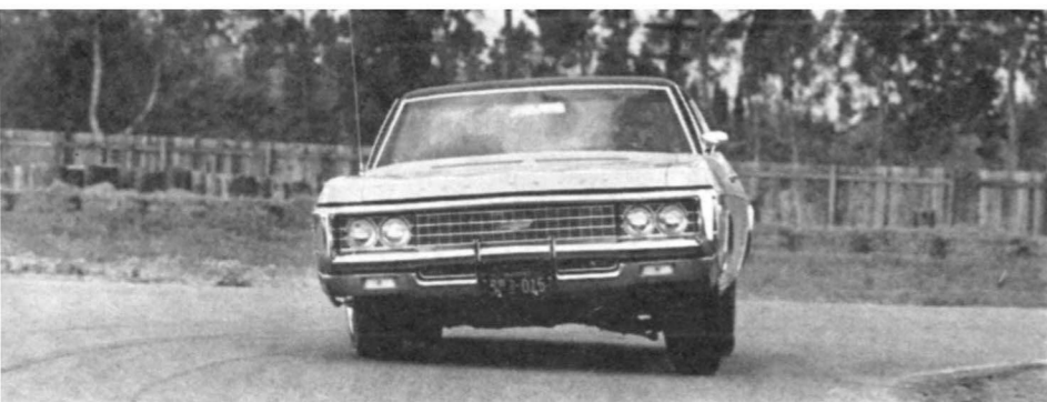
ROUNDING 40-mph test curve at target speed, the Caprice displayed mild understeer and moderate body lean. More power produced neutral steer.
