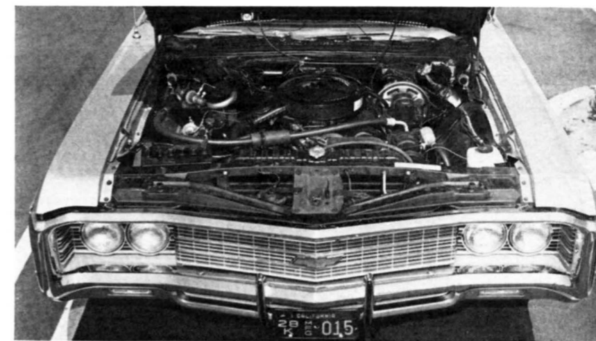
BIG ENGINE is all but lost in the big engine compartment. The 390-bhp/427-cid V-8 delivered plenty of performance and acceptable gas mileage.
