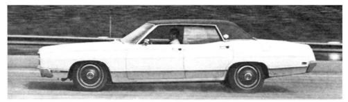
PROVERBIALLY GOOD Ford brakes came through once again. Consistent deceleration rates at 28 ft./sec./sec. were recorded with no fade evident.
