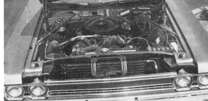
SMALLEST engine among the Powercars tested was the Fury's 383-cid V-8. Lack of inches did not hurt it at all.
