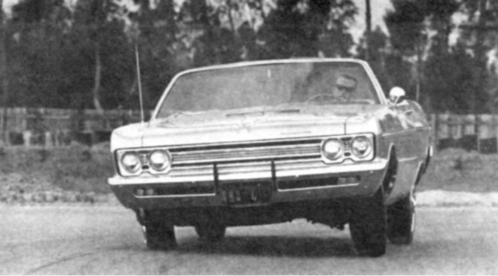
CORNERING in tight, 40-mph bend, caused Fury to tuck under its outside wheel and plow.
