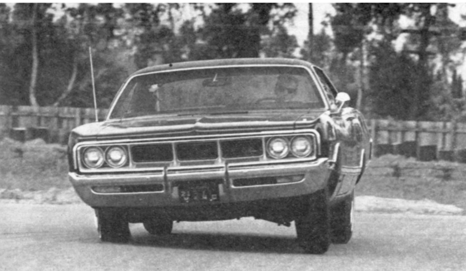
STRONG FAMILY resemblance between the Fury and Monaco is demonstrated as the Monaco plows around the 40-mph test corner. Understeer was controllable.
