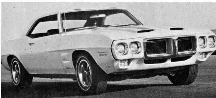
Functional twin-scoop setup directs cool fresh air to the hungry 400 Ram Air mill.
