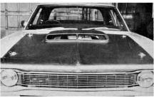
New Coronet setup makes use of the best available California and factory speed equipment. The aluminum manifold is from Edelbrock, while the fresh air induction system is straight from the factory. The carbs are Holley units specially jetted for the ram-air kit.
