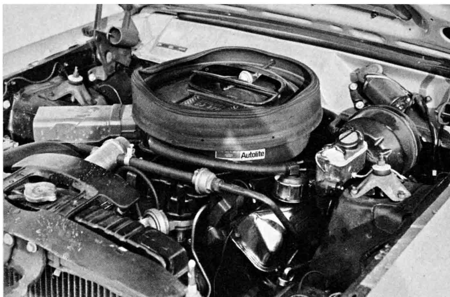
Hidden under the huge air cleaner, smog controls and PCV rests a 428 monster mill.
