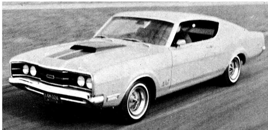
Hot Cyclone CJ is stable at high speeds and tracks well considering compromise suspension.
