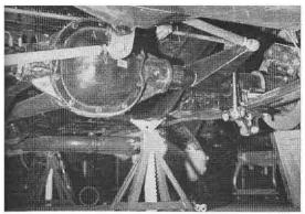
Rear axle (above) is controlled by familiar Watts-link mounted on frame instead of axle to reduce unsprung load. Delco-Moraine discs are used all around with Koni adjustable shocks. 'Bird's frame was stiffened with bridge-truss (top) and roll cage (right). Superior Prod. wheel, S-W gauges are used. Anticipating the season, Jerry Titus (opposite page) bridges street/track cars.
