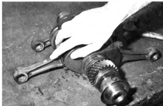
To mount the rods right, lay the crank down and insert the rods in order, making sure this little mark faces upward.
