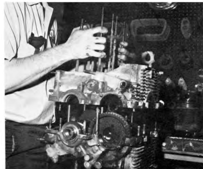
With everything removed and the bolts loosened, Dunerod's case was split and the inner workings of the German masterpiece were revealed.
