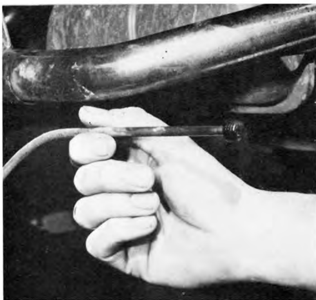
A time saver: the rubber cap on the brake bleed fittings will fit snugly over the gas line to seal it after disconnection.
