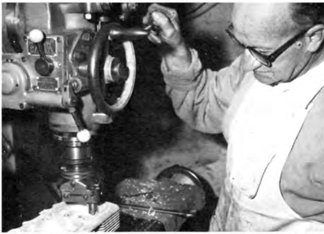
George Beavis cut .338-inch from the head combustion chamber's diameter to fit our new larger barrels.
