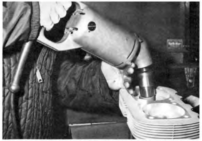
With the machine work complete, John reground our valves and valve seats and did a stock-type valve job.
