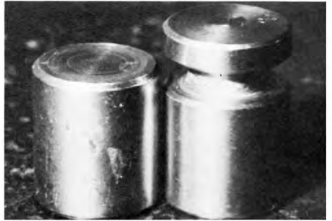
A new longer oil pressure check valve (right) was installed into the Dunerod for a 30 per cent cooling increase.
