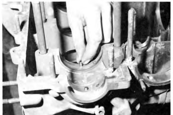
Small dowel pins in the case match with holes to the rear of center in each main bearing to locate the bearing.
