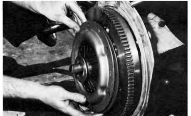
A new heavy-duty Scat diaphragm clutch was installed to handle our refurbished powerplant. The first clutch engagement showed the benefit of this larger unit.
