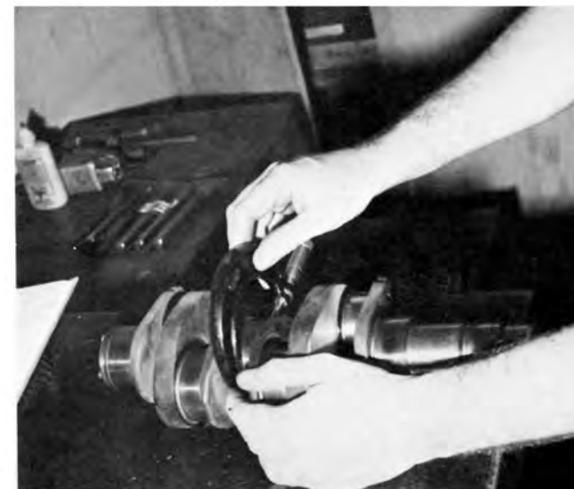
First indications of our engine's good condition came when a micrometer check and a check for straightness showed our crank to be in near new condition.
