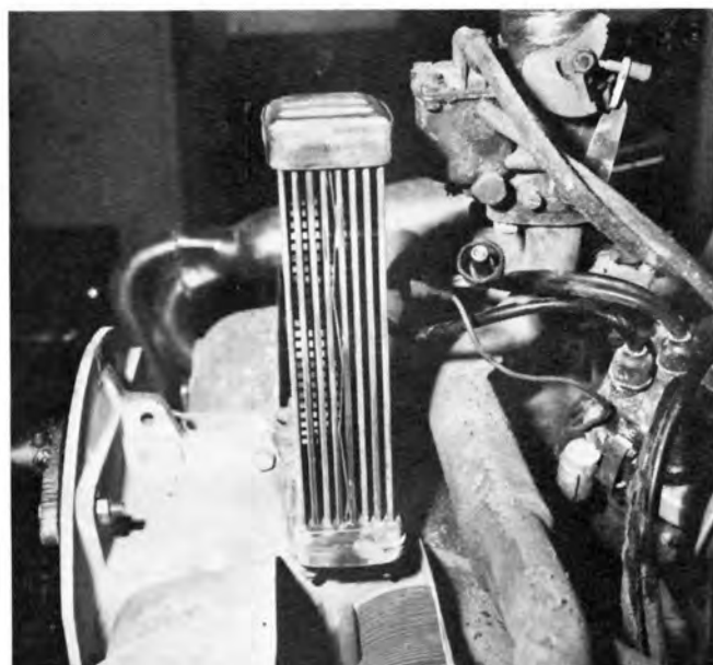
Under the main fan shrouding is the oil cooler. This will often cause an overheating due to a dirt buildup. This is the first place to check whenever overheating is a problem.
