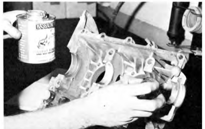
No gasket is used between the case halves, so a coating of gasket sealer is applied for a tight seal.
