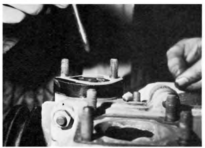
This fuel pump pushrod, inserted through a plastic guide block, must go into the engine pointed end first.
