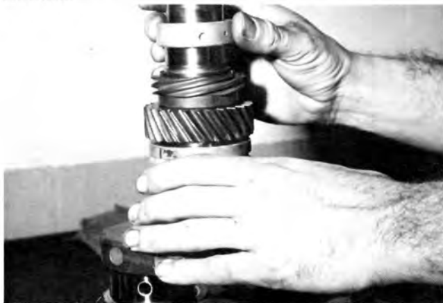
When replacing main bearings on the crank, the dowel pin locator holes go towards the engine's rear.
