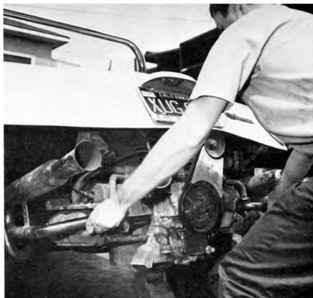
For engine removal, a floor jack is handy, but two people can easily lift the aluminum VW powerplant out of the car.
