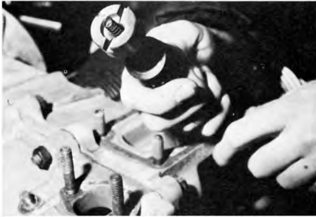
The slot on the top side of the distributor drive gear must be towards the front or pulley end of the engine when installed.
