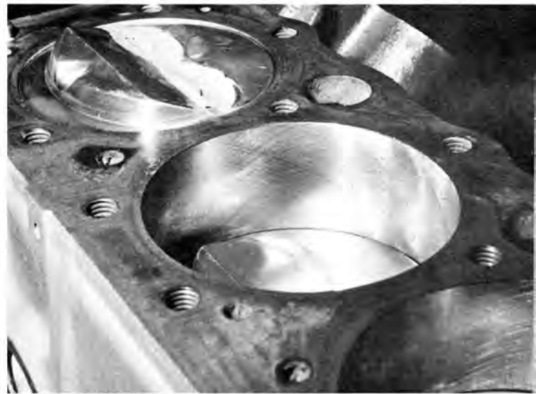
One trick is the cylinders hone. A 45-degree crosshatch pattern is used. The rougher the hone the quicker rings seat and wear out. Ramco Piston Rings are used on JE Pistons.
