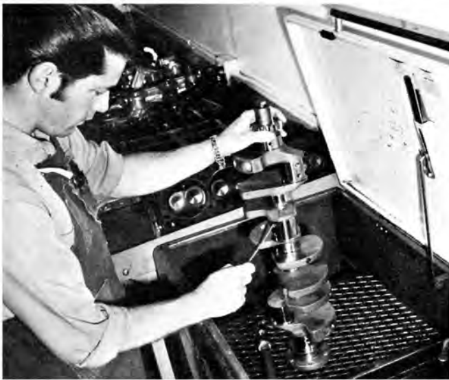
Cleaning the CrankShaft Company crank is done with a special brush to get inside the oil passages and radii. Only clean solvent is used here.
