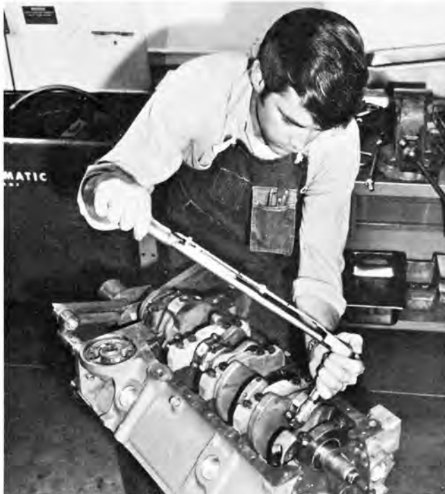
Torque on the bolts, of course, is important. Bring torque up gradually until exact readings are obtained.
