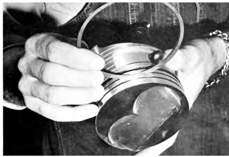
Ring depth must be checked to assure proper fit. If ring sinks below ring land groove then depth is okay.
