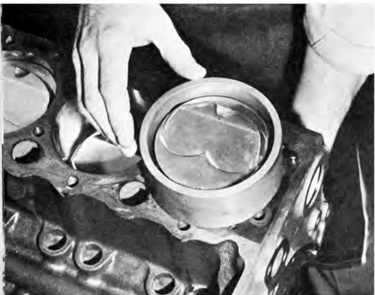
The JE Pistons are put into place after special attention to the piston and rod assembly has been carried out. Ring compressor used is manufactured by Pink in all bore sizes.
