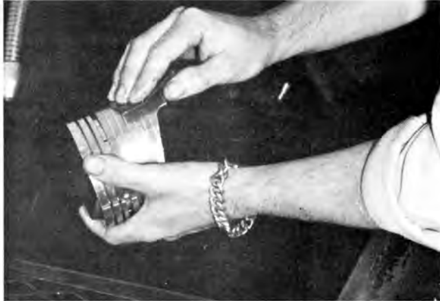
Lightly sand the pistons with a 320 or finer grit of wet and dry sandpaper.
