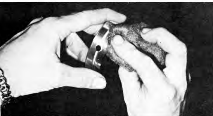
Debur the bearing carefully and then lightly buff the surface with a "000" grade of steel wool.
