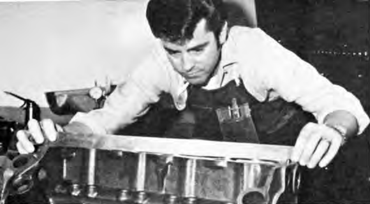
The blocks deck (top surface) is checked by the "young master", Larry Dixon, to see if there is evidence of uneven surfaces.
