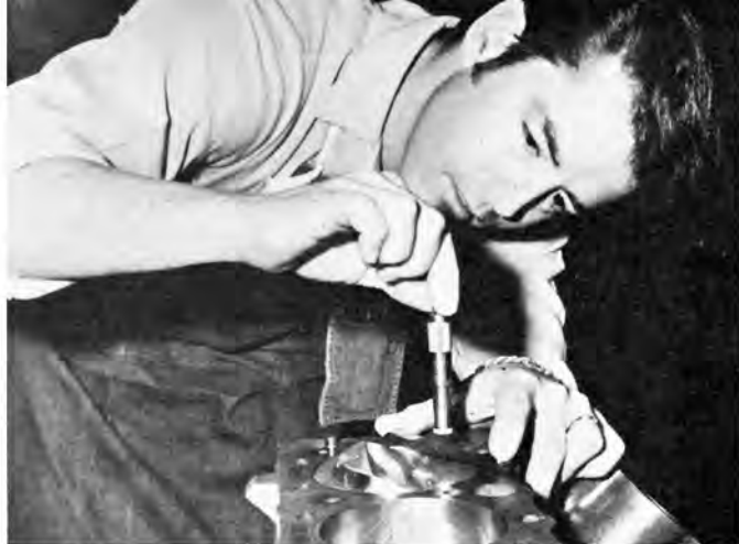
The actual deck is determined by micrometer checks of each piston in the cylinder. The average here was .018. Your deck height is a determining factor for compression ratios.
