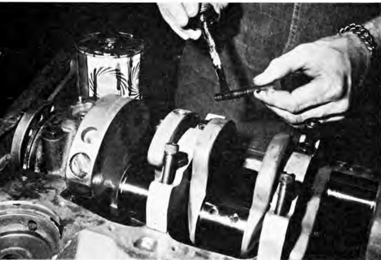
A major change to the engine's lower end was the addition of Summers Brothers Engineering four-bolt main caps. Sealer is used on the outside bolts as they enter the water jacket. Special block surfacing should be done prior to installation.
