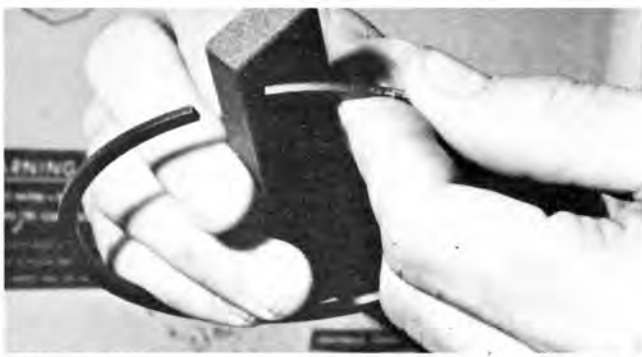
Ring edges are deburred with a fine grit stone. Eliminates snagging in the ring groove.
