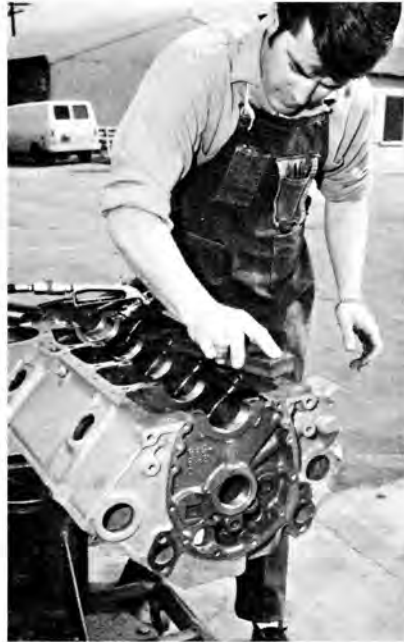
Cleanliness is the name of the game. Brushes and solvent are used in the bores, oil passages and all surfaces and then soap and water are used to remove all particles. The decks are lightly burnished with a stone from machine work.
