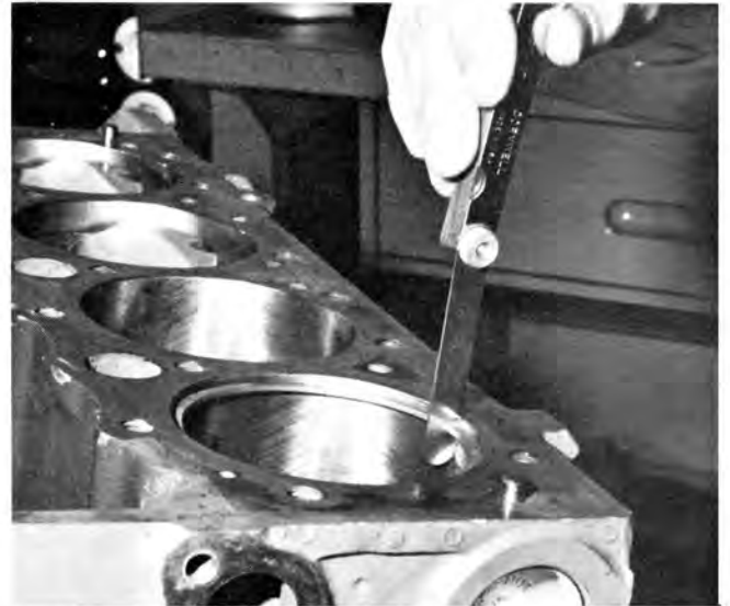
Butt clearance is measured with feeler gauge: Preferred clearance is .024-to-.028.
