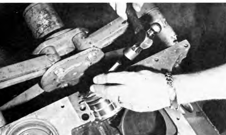
The rear oil main seal groove is center punched extensively to prevent the carbon rope seal from spinning.
