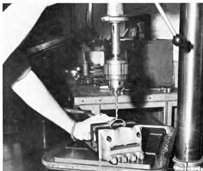
Again a trick! Drill the oil passage holes out to the same size as those in the block.
