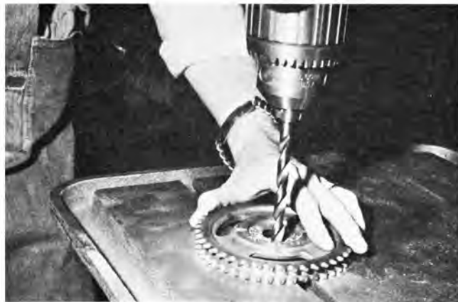
A dual chain timing gear sprocket is used in place of the stock single chain unit. Here, holes are being drilled out so offset bushings can be used to bring cam timing to desired specs.
