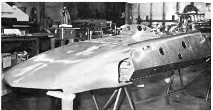
Wedge shape design of Gurney Eagle features a wider, lowered car with better weight distribution.
