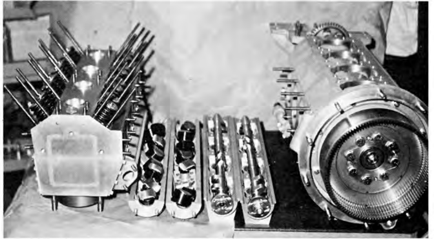
Offenhauser engine components ready to be assembled for use in an Indy race car. Cylinder block is aluminum with water side plate. Valve tappets and cam cover, cam housing and two cams are in center, while American Borg & Beck three-plate clutch for flywheel is shown with crankcase at right.
