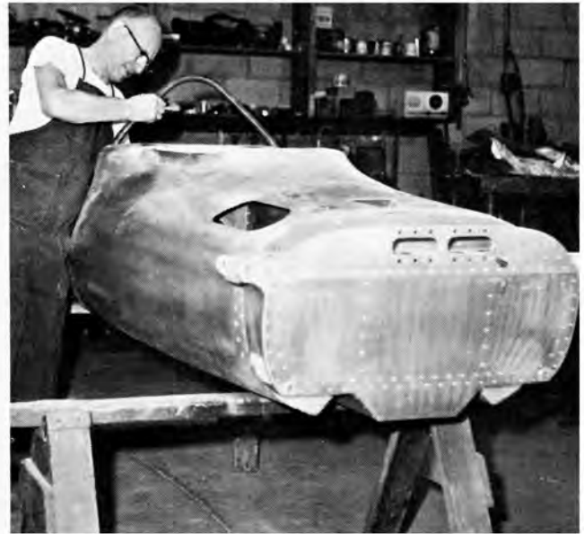
Eddie Kuzma, builder of race cars for A. J. Foyt, is shown with body-chassis of car being constructed for Indy. Bulkhead is steel, body skin is .063 aluminum and roll bar is one-inch chrome moly with 1/8-inch wall thickness.
