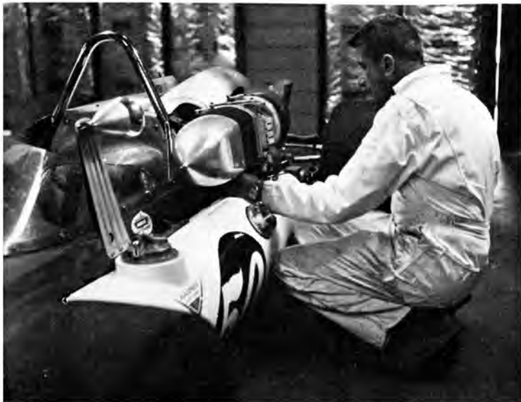
Barney Navarro, whose hot rodding activities go back to the dry lakes racing days, checks the injection system he designed for use with the AiResearch turbo-charger unit on race car he's entered at Indy.
