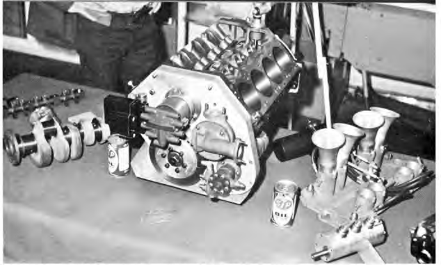
Components of Plymouth's stock block V-8 passenger car engine, 318 cubic inches, are displayed at STP headquarters for magazine writers. STP is experimenting with both Hilborn and Bosch injection systems.
