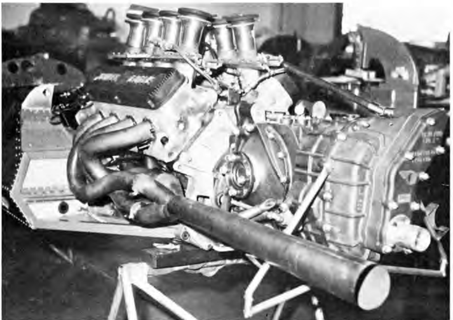
Displacement of Gurney Eagle Ford engine has been increased to 320 inches, maximum for American stock block powerplants under new Indy rules. Rear end is Hewland unit.
