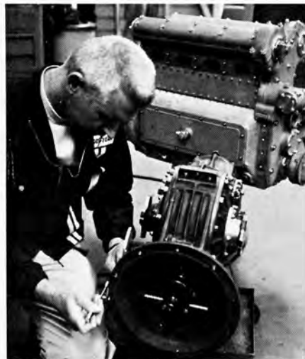
Halibrand rear end gets adjustment from race car builder A. J. Watson before being installed in car to be driven by Mike Mosley. Offenhauser engine, in background, will power car entered by Leader Card Racers.
