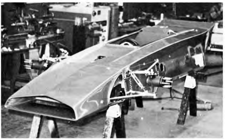
Aerodynamic wedge shape design to create negative lift is shown on the full monocoque chassis of car built by Eisert Racing Enterprises for owner Lindsey Hopkins and driver Wally Dallenbach. Spoiler has four-inch angle. Car has five-speed Hewland gear box.
