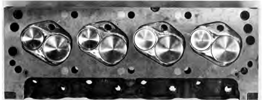
New stagger-valve arrangement and improved combustion chambers on Ford's 302 small-block may mean a reversal of last year's dismal showing on Trans-Am circuit. First reports say that the new 302 really wails!
