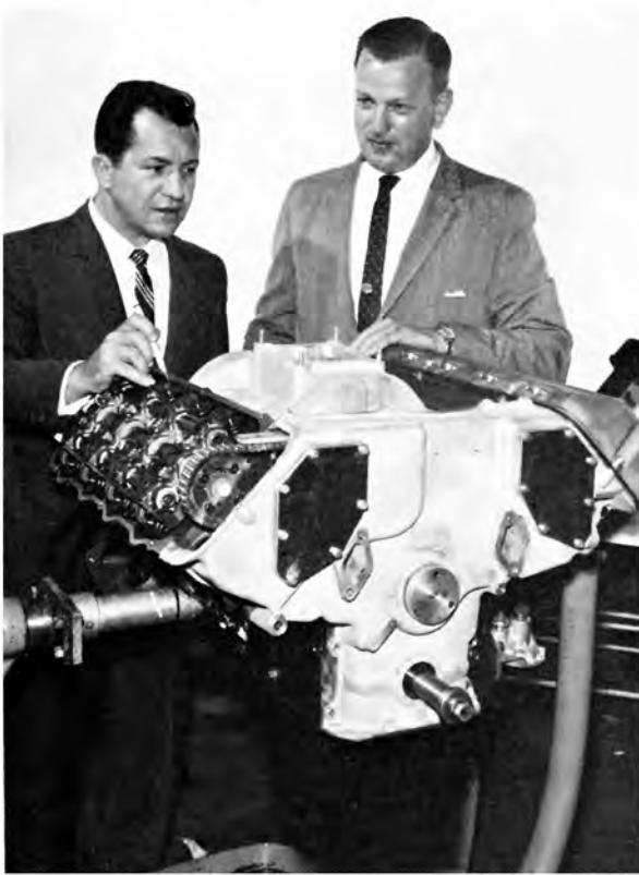
Norm Faustyn (left) and Joe Eastman were top project engineers on the overhead-cam 427 project. Special heads and front end chain cam drive adapted to standard 427 NASCAR block, giving over 600 hp at 7200 rpm in an engine that could sell for $3000.
