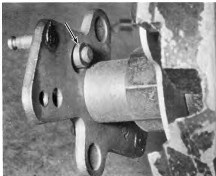
Total centrifugal advance (limit) can be regulated by change of shape of stop-bushing (in GM type distributor shown). Limiting rate and total amount of centrifugal advance can provide room for additional crankshaft timing boosts, resulting in improved low rpm response and economy without attending over-advance when rpm surpasses limit of centrifugal advance.
