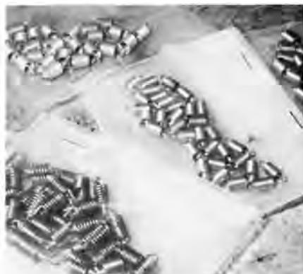
*Assortment of centrifugal advance springs permits various tailored advance curves of equally as assorted engine applications. Stretching or loop-clipping of stock springs helps, but use of special spring designs often provides best curve shape and resulting ignition performance.*
