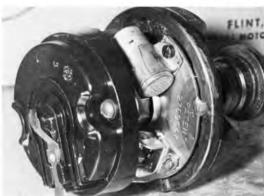
*Point plate wobble is a definite problem with many stock (and modified stock) distributors. To cure the ailment, you can tack-braze the point plate to the housing, eliminating wobble and attending timing and point dwell variations (for distributors not incorporating vacuum advance mechanisms or those whose vacuum units are disconnected).*
