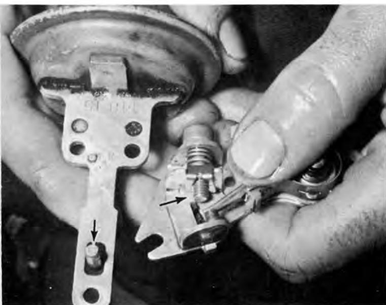
Vacuum advance control is simple feature if you'll construct adjustable arm as shown. Simply trim the adjustable spring-loaded ignition point pad from a set of GM points, tack-braze this cutoff section onto the bottom side of a stock vacuum advance plunger arm guide (the flat strip section) and use the screw stop to limit advance movement of the diaphragm plunger rod. Limitation of rod action permits increased crank lead (initial timing) without total disruption of fuel-saving vacuum unit.
