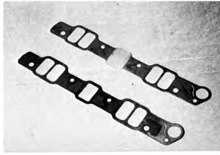
Special blocked heat riser intake manifold gasket aids performance in warm weather but should not be used in colder climates.
