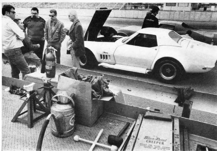
DUNTOV TO EDITORS and bystanders during rain break: "We did what a man would do on his own" by removing everything from a Corvette that doesn't look like a racing car. (Lip on leading edge of hood is to hold hood on above 180 mph.)
