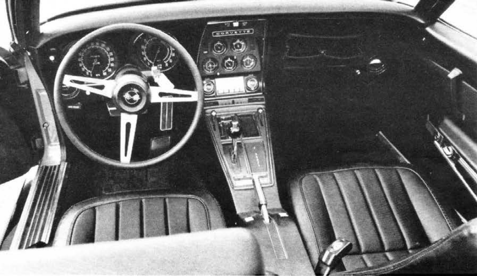
COCKPIT DESIGN works with big, legible instruments, good seats and controls within reach. Four-speed gearshift, right, is one of the best factory-built shifters out.
