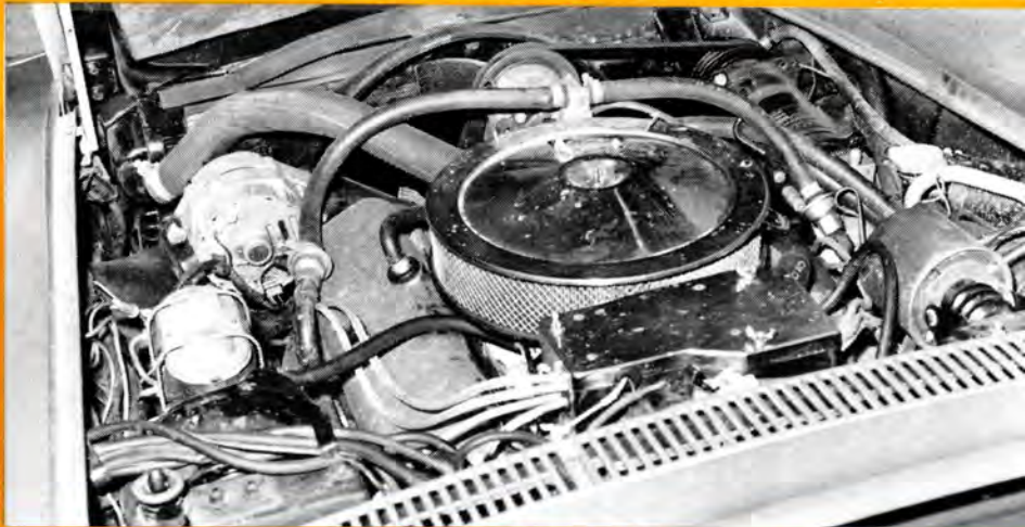
BIG CORVETTE engines come in a wide assortment. Directly below is the L36, the understressed base for the 427-cid range. At lower right is the L89, the hottest street Corvette. It looks like the L71, same engine with aluminum heads or the L68, same triple carburetors but the camshaft from the L36. At bottom left is the L88, with cold-air air cleaner and a huge four-barrel carb.
